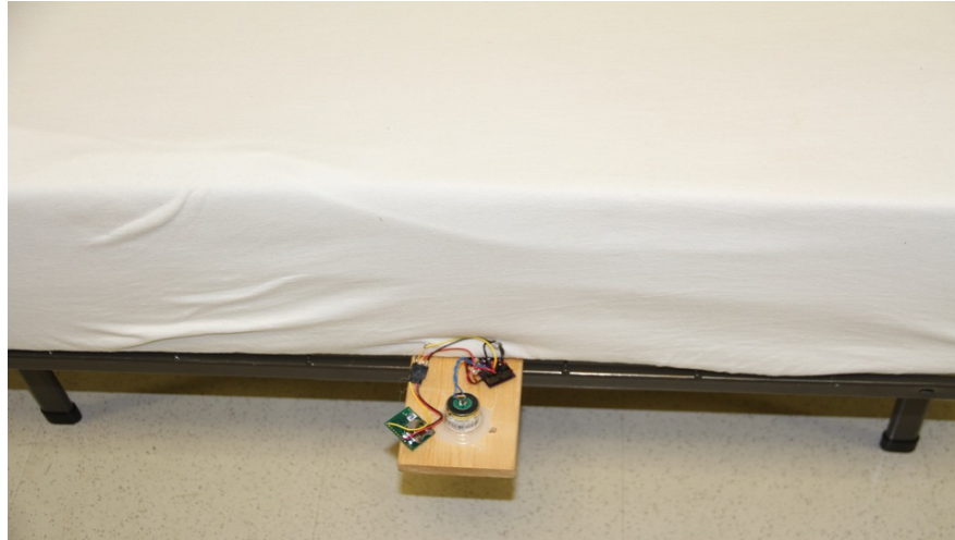
Figure 5.4: The picture of our MotionPhone prototype, where the geophone, the amplifier, and the PIP-Tag are attached to a wooden board that is inserted between mattress and bed frame.
