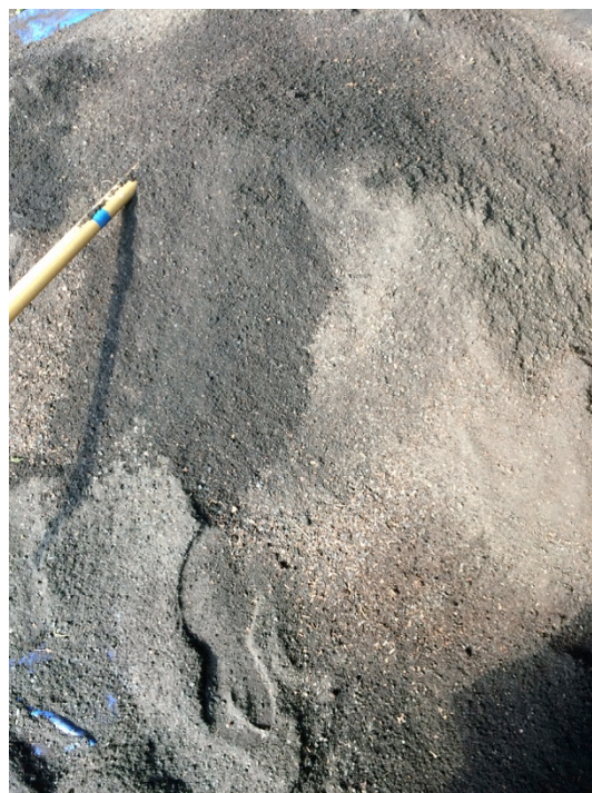
Figure 3-5: Polluted soil from Liberty State Park. Note extreme color differences indicating differing pollution levels (size 12 shoeprint for scale).
