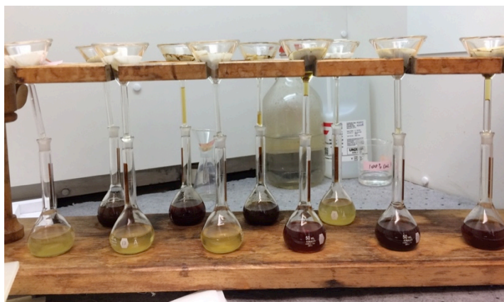
Figure 3-9: Volumetric flasks and filtering apparatus for processed analytes.
