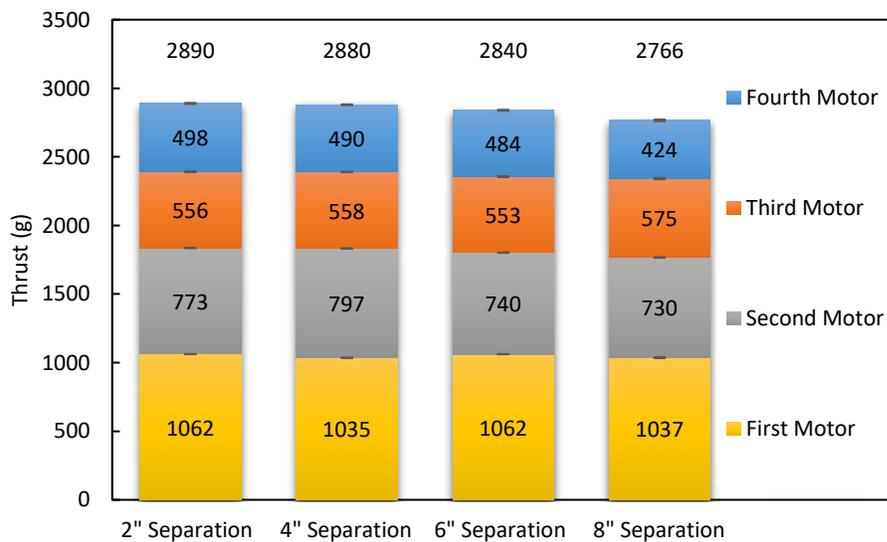
**Figure 21.** Separation distance was altered and the experiment associated with Figure 7 was repeated. Between two and eight inches of separation between propellers’ planes of rotation, little change is observed.
