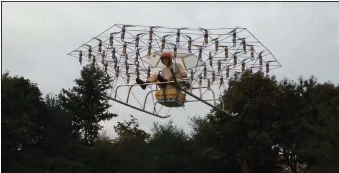
**Figure 2.** YouTube user gasturbine101's The Swarm is a proof-of-concept electric passenger multirotor aerial vehicle.
