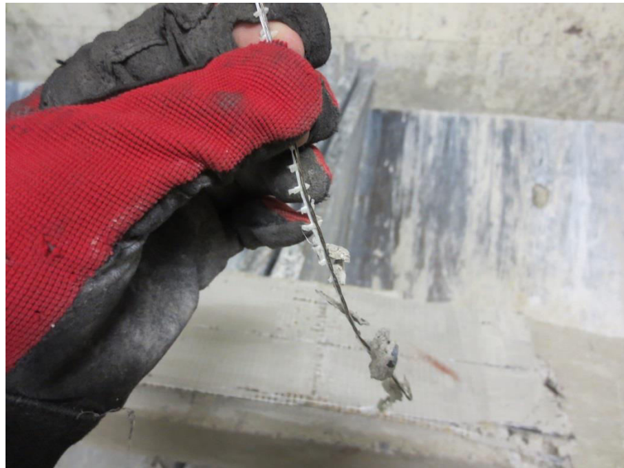
Figure 4.12 Brass Coating No Longer on Steel Strands
