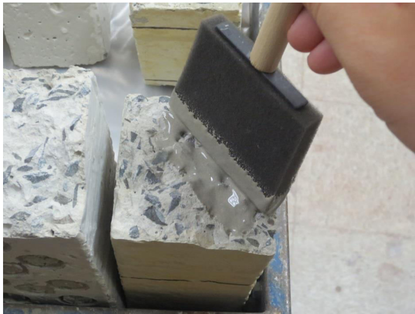
Figure 3.12: Application of geopolymer matrix for Flexural Repair testing
