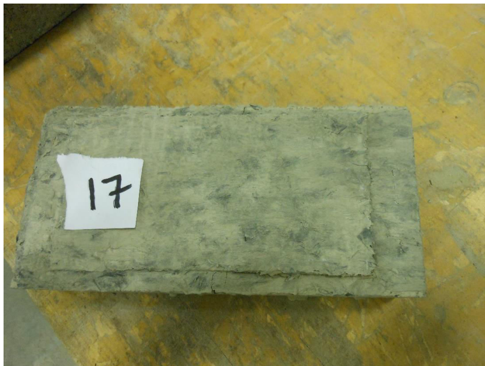
Figure 3.5: Hand Mixed Carbon Fiber Sample
