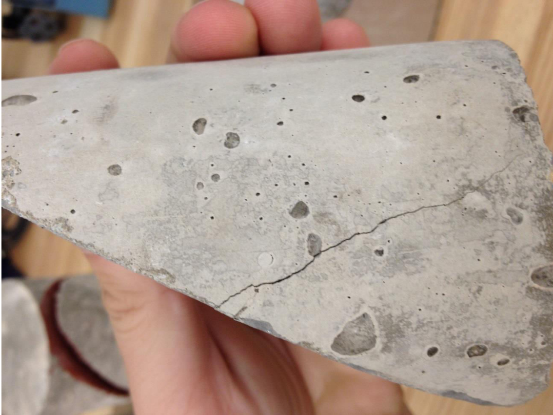
Figure 3.23: Failure through concrete in secondary slant shear testing
