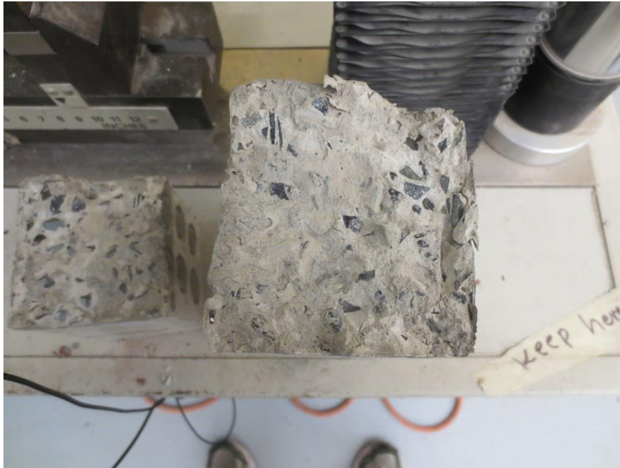
Figure 3.15: Flexural failure through both repair matrix and concrete
