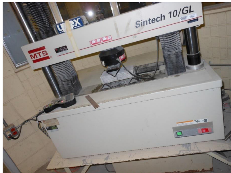
Figure 3.7: Testing Setup for Flexure of Reinforced Brick Specimens
