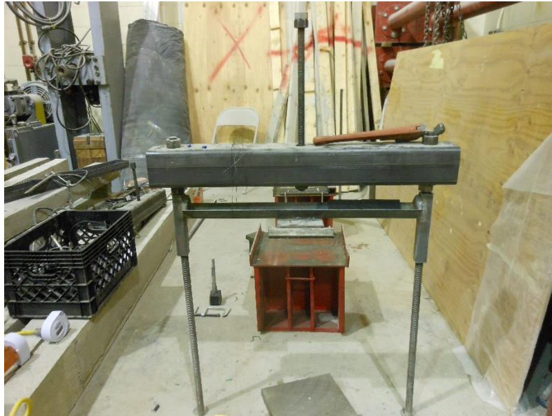
Figure 5.3: Loading apparatus for heat testing rig
