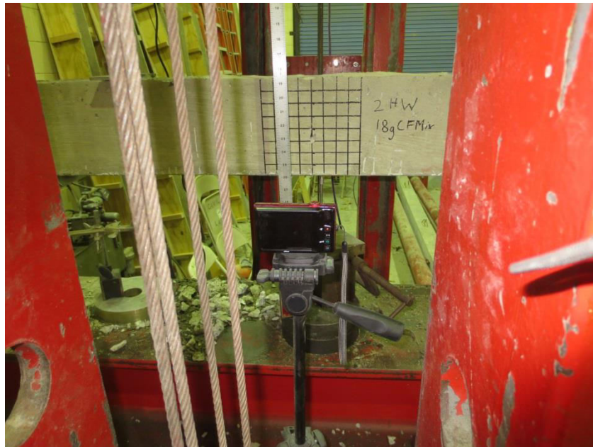
Figure 4.9 Additional Deflection Recording
