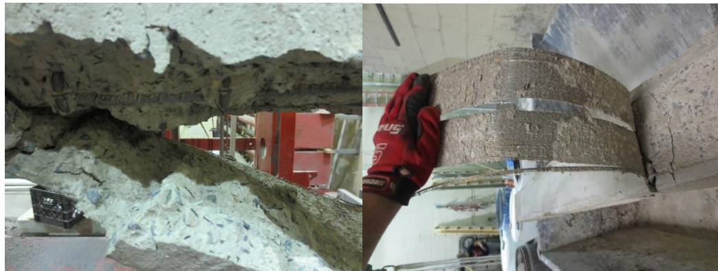
Figure 4.11 Levels of Concrete Pull Off in Beams
