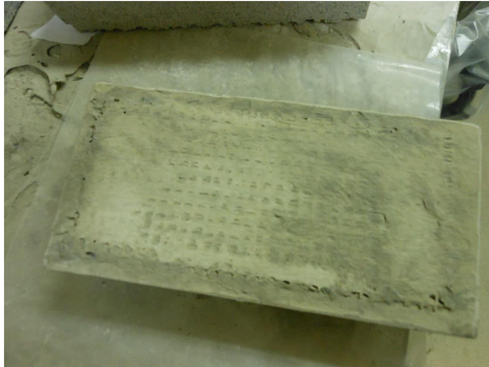
Figure 3.3: Reinforced Concrete Brick Sample
