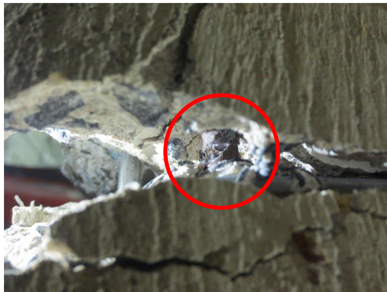
Figure 4.10 Ruptured Tension Bar in SRiP Control Beam
