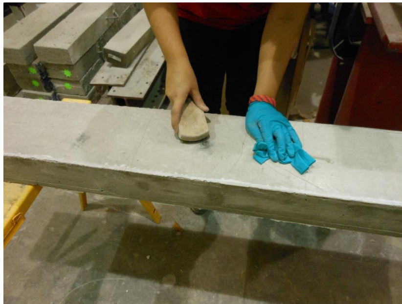
Figure 4.3 Cleaning with a handheld wire brush before application
