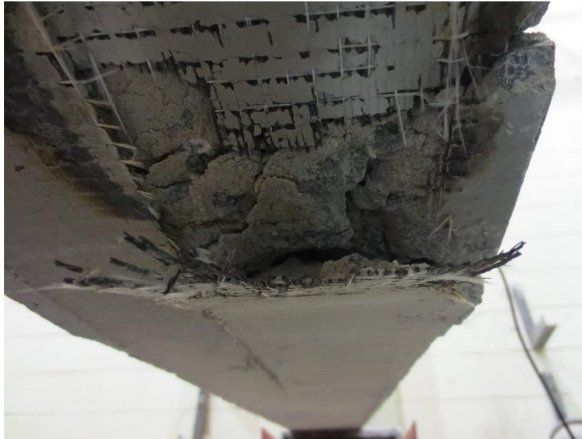
Figure 5.16: Damaged Hardwire Backing
