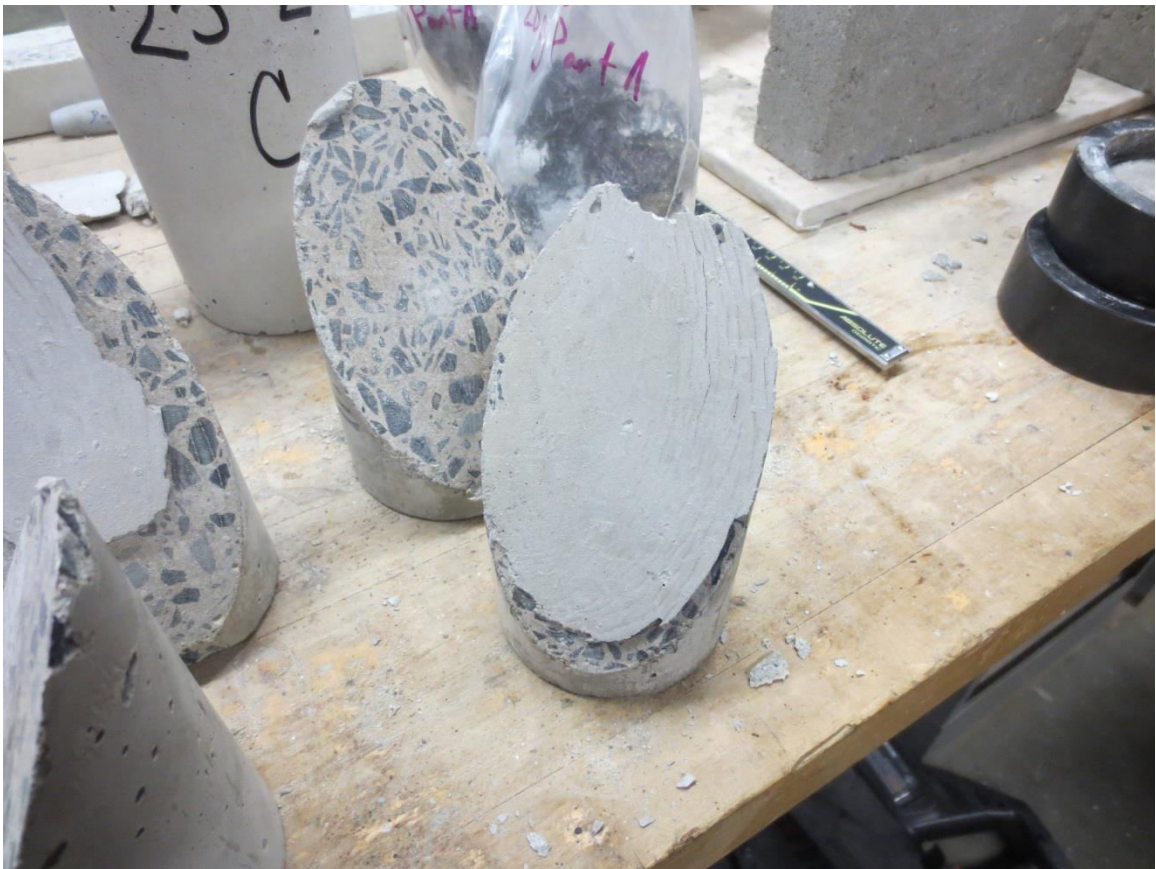
Figure 3.22: Initial slant shear testing with smooth failure at repair site
