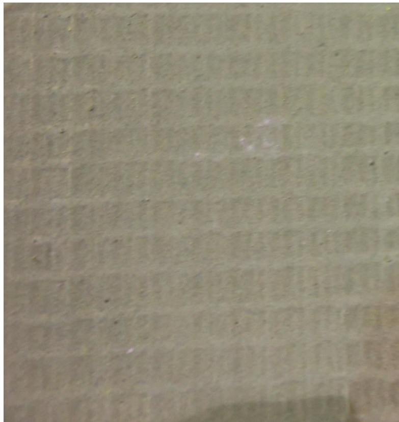
Figure 3.6: Blender Mixed Carbon Fiber Sample
