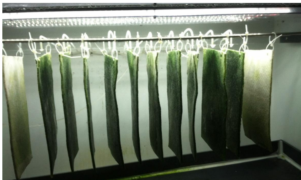
Figure 2. Small scale aeroponic substrate based system which was inoculated with P. kessleri and irrigated for three weeks. The left most and right most substrates are not inoculated or irrigated and serve to maintain consistent lighting amongst all ten growth substrates. At the top of each substrate a small 1/8" irrigation dripper can be seen and the nutrient solution that drips off the bottom of the substrates is collected and used for analysis. The substrates are contained within a closed chamber and are illuminated with an array of LED lights on a 16 hour on and 8 hour off light cycle.
