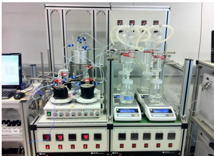
**Figure 2.1.** An experimental set up used for measuring volume of  $\text{H}_2 + \text{CO}_2$  (mL).
