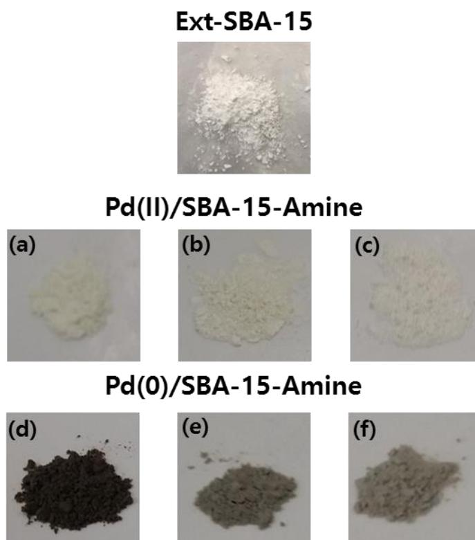
**Figure 3.2.** Photographs of Ext-SBA-15 (1<sup>st</sup> row), Pd(II)/SBA-15-Amine (2<sup>nd</sup> row), and Pd(0)/SBA-15-Amine (3<sup>rd</sup> row). (a) Pd(II)/SBA-15-PA, (b) Pd(II)/SBA-15-SA, (c) Pd(II)/SBA-15-TA, (d) Pd(0)/SBA-15-SA, (e) Pd(0)/SBA-15-SA, and (f) Pd(0)/SBA-
