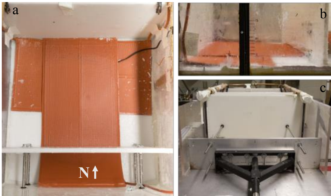
Figure 6: Experimental apparatus box set-up, with overhead, cross section, and moving wall coupling views. (a) Overhead view, (b) side view (looking east), and (c) moving wall couple. Note: orange heat mat array in (a), (b); scale on the side wall in (b); and U-shaped copper cooling manifold at the top of the box of (c).
