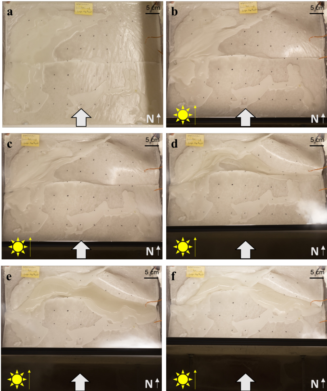
Figure S: Map view of 2 cm thick solid layer deformed at 30 cm/hr., inclined PZW at a) initial conditions, b) 2 cm displacement, c) 4 cm displacement, d) 8 cm displacement, e) 10 cm displacement, and f) 13 cm displacement. Lightning directions and symbols as in Fig. A.
