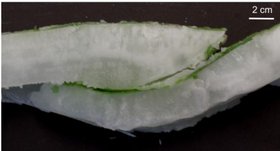
Figure 8: Example of a cross-section view (looking west) of a typical subsumption experiment. The thin green layer is colored wax painted onto the experimental wax surface before the onset of boundary displacement. Inclined PZW, 30 cm/hr. boundary displacement rate. Total boundary displacement was 13 cm.
