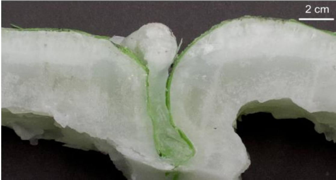
Figure 9: Example of a cross-section view (looking west) of ductile roll back experiment. The thin green layer is colored wax that was painted onto the experimental wax surface before the onset of boundary displacement and traces the path of ductile roll back. Wax between both plates upwelled during PZW cut. Vertical PZW, 1 cm conductive layer thickness, 30 cm/hr. displacement rate. Total boundary displacement for this experiment was 13 cm.
