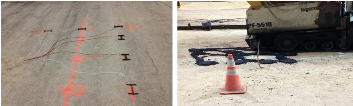
Figure 6.2 Pavement instrumentation: (a) layout and (b) protection of asphalt strain gauges
