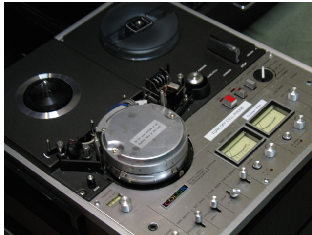
Figure 9 – Color ½" Open Reel Video Tape Recorder (VTR) (Digital Photo Taken by Author at Site L2)
