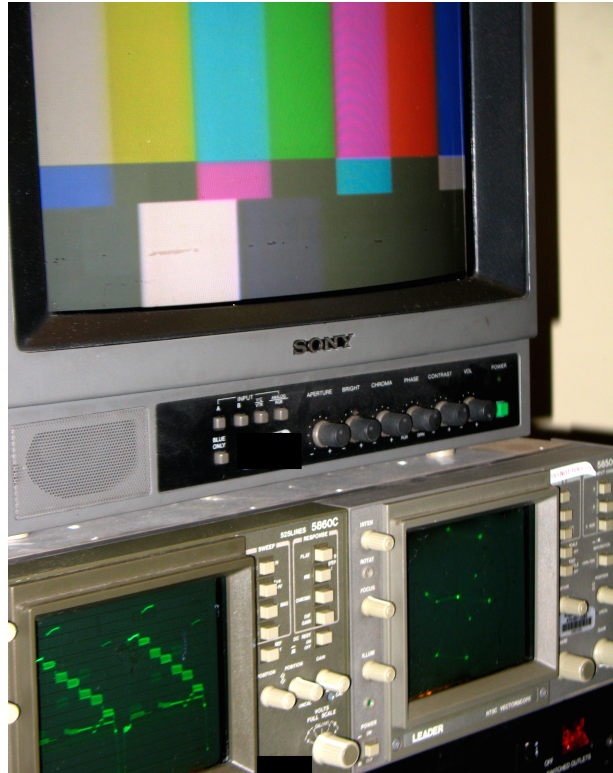
Figure 10 – CRT Monitor (Top) Waveform Monitor (Left), Vectorscope (Right) (Digital Image Taken by Author at Site L2)
