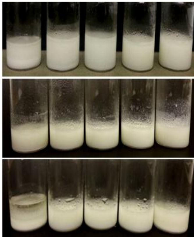
Figure 7. Vessels containing Pickering emulsions stabilized by three different milled starches after 2-month storage at different milling times. From left to right: 5 h, 10 h, 15 h, 20 h, and 25 h (milling time). From up to down: normal maize starch, high-amylose maize starch, waxy maize starch.
