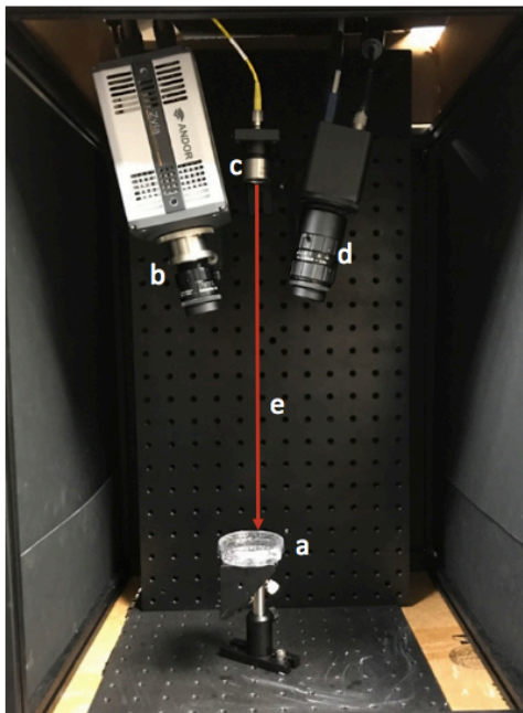
Figure 33: The set-up used to image visible and SWIR wavelength emissions from rare-earth-doped nanoparticles. A 980 nm collimated beam was used to excite the nanoparticles, while the silicon camera and the InGaAs camera simultaneously captured emissions. (a) Nanoparticles (b) silicon camera (c) 980 nm collimated beam (d) InGaAs camera. The setup was enclosed in a light tight box.
