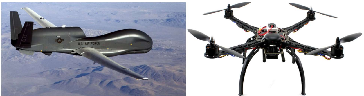
Figure 1.1: Examples of Fixed-Wing and Quadrotor UAVs (a) The Northrop Grumman RQ-4 Global Hawk Fixed-Wing UAV [14], (b) The Storm RC Hobby 550 mm RTF Quadcopter UAV [15].
