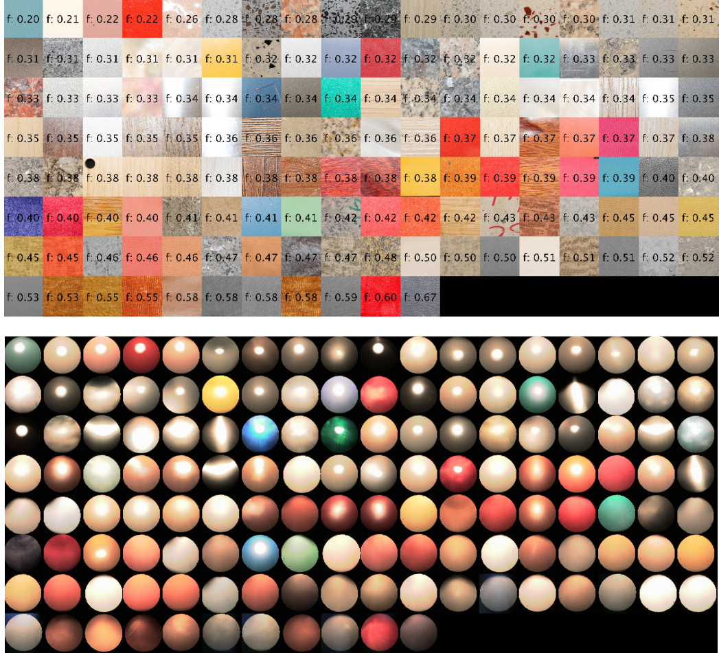
Figure 3.2: (Top) Images of the 137 material surfaces for the friction-material database ordered by friction coefficient. (Bottom) Example reflectance disks for corresponding material surfaces. The names for all material classes and the number of instances captured per class are shown in Table 3.1. As examples of material class names, the list of names for the first surface in each row are as follows: Smooth Ceramic Tile, Automotive Paint, Marble, Composite Flooring, Asphalt, Nylon, Linen, Leather and Sand Paper. As expected, samples such as Smooth Ceramic Tile have lower coefficients of friction (0.2) than samples such as Sand Paper (0.53).
