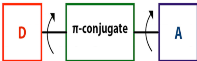
Figure 2.9: Schematic diagram of molecular rotor structure that adopts an “electron donor- \pi -electron acceptor” (A); ‘D’ represents electron donor segment, ‘A’ represents electron acceptor segment; the two segments are connected via a \pi -conjugation unit. Adapted from Haidekker and Theodorakis [231].
