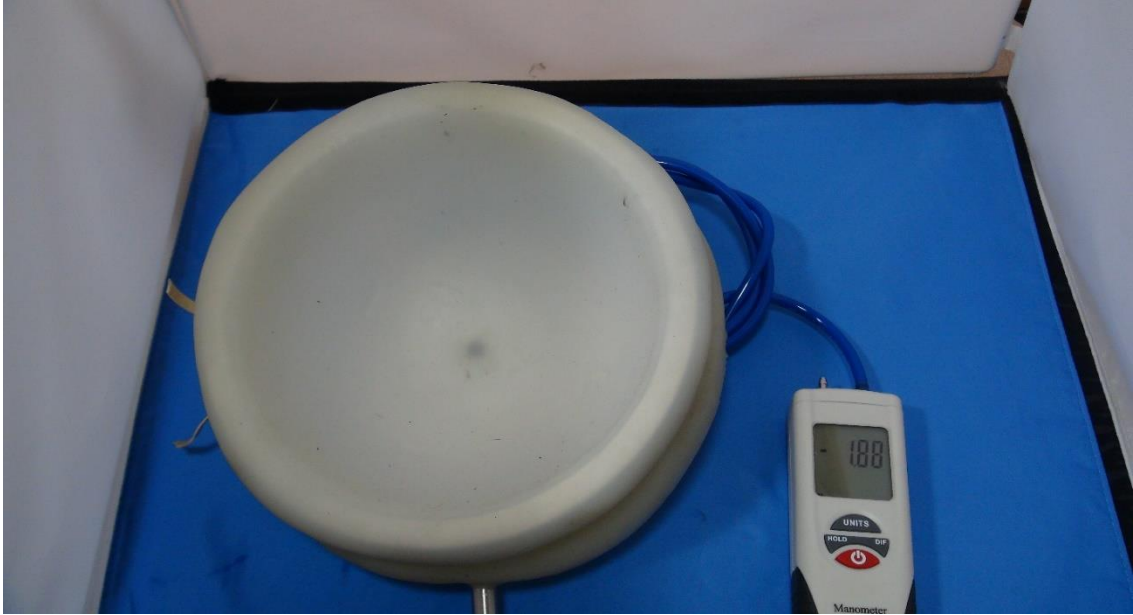
Figure 4: Digital U-tube manometer to measure vacuum inside the reflector assembly. We keep one end of the manometer exposed to the atmosphere. The manometer indicates differential pressure in (-kPa). The manometer has the options to record and switch between unit systems.
