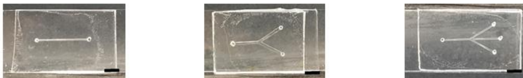
Figure 2.11: Fabricated PDMS Microfluidic channels. Scale bars 5 mm.
