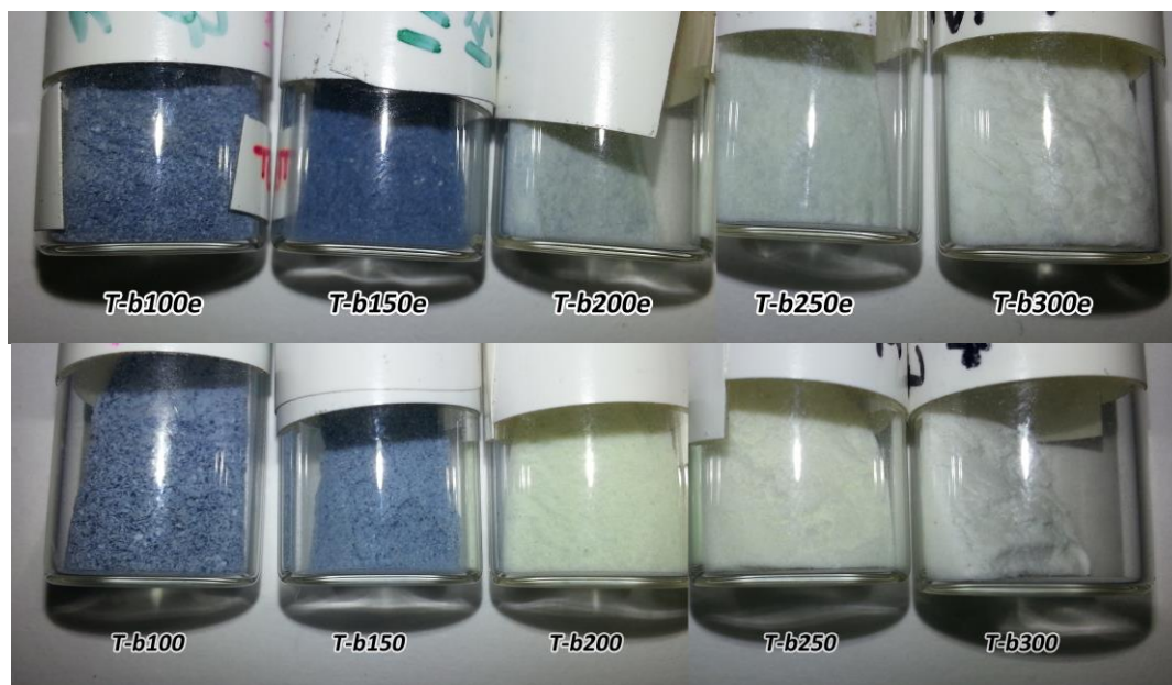
Figure 12 Collected powders indicating observed differences between the impinged area (bottom), and the rest of the covered plate. For this thesis, we focus on the center samples
