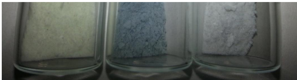
Figure 13 Optical image of Tb-250, Tb150 and Ta150 (left to right). Note not white appearance of Tb250 and Tb150, indicating visible color absorption and signs of doping.
