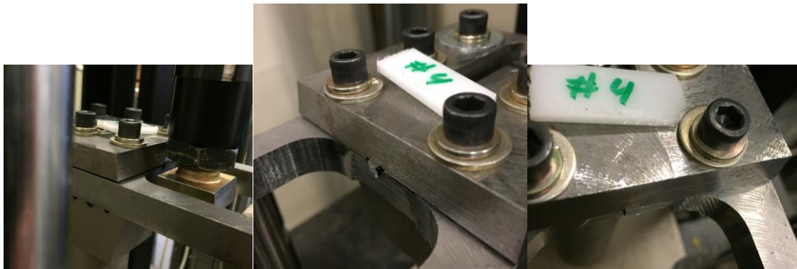
Figure 6.2.4 Posttest Pictures of Specimen 4 Impact Testing
