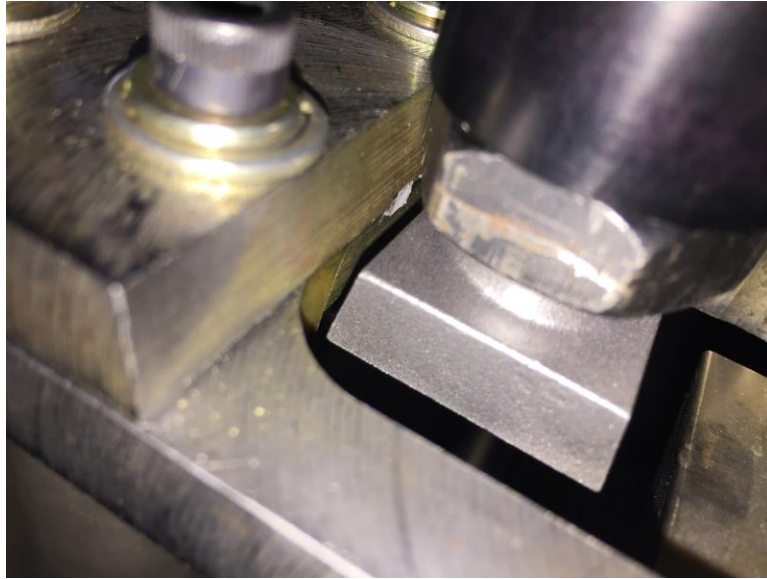
Figure 6.3.2 D2 Impact Testing Sample 5 Hardened Striker
