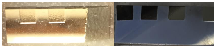
Figure 2.2.1 WHA in D2 Polished Sample (Left) Etched Sample (Right)
