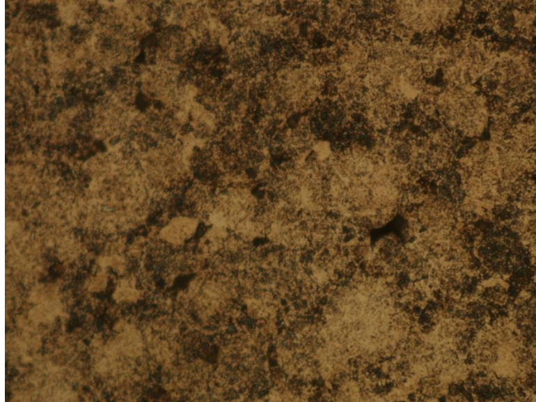
Figure 2.2.20 Etched D2 Between WHA Cubes Showing Martensite and Ferrite 1000x
