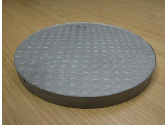
Figure 2.1.6 D2 and WHA Composite Manufactured with FAST
