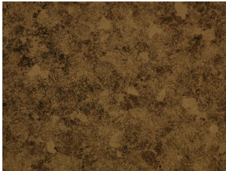
Figure 2.2.17 Etched D2 Showing Martensite and Ferrite 1000x
