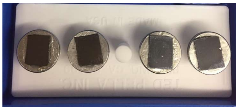
Figure 3. 4: Melting gel (oligomeric silsesquioxane polymer) specimens glued on SEM pucks with CA glue.
