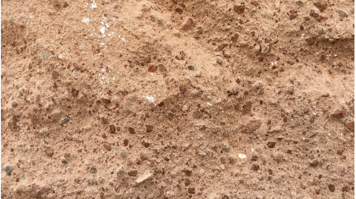
Figure 13. Mortar, containing smaller stone fragments and broken red clay bricks. Source: Author Image
