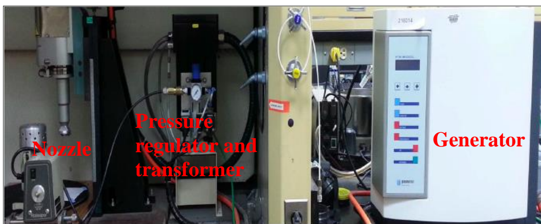
Figure 9: Cold Atmospheric Plasma Processing Unit (Plasma Treat Inc., Elgin, IL) for generation of PAW at the Department of Food Science, Rutgers University.
