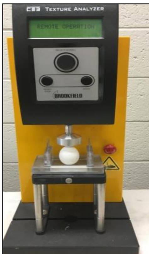
Figure 12: CT3 Brookfield Texture Analyzer at the Department of Food Science, Rutgers University with custom designed aluminum probe and farm egg at the Small end up position.
