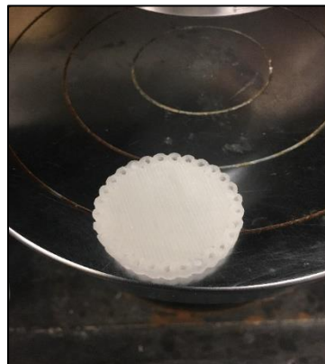
Figure 30: The whole scaffold with two hydroxyapatite posts used for compression testing.
