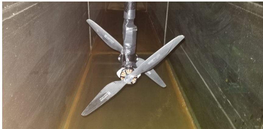
Figure 6.4: Picture of the experimental setup for collecting data corresponding to the thrust produced by a pair of counter-rotating coaxial rotors placed inside of a water channel in preparation for static and dynamic water testing.
