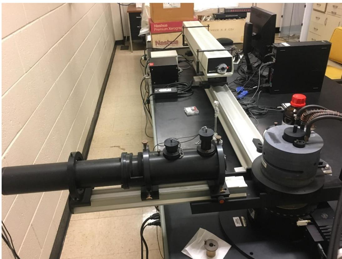
Figure 1.3: Dynamic light scattering instrument
