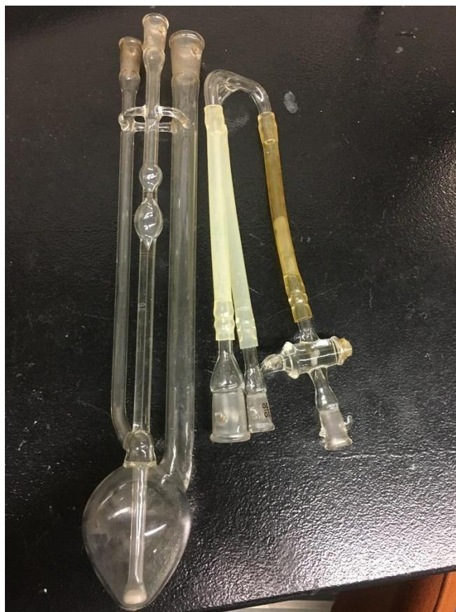
**Figure 1.2:** Ubbelohde Viscometer[35]
