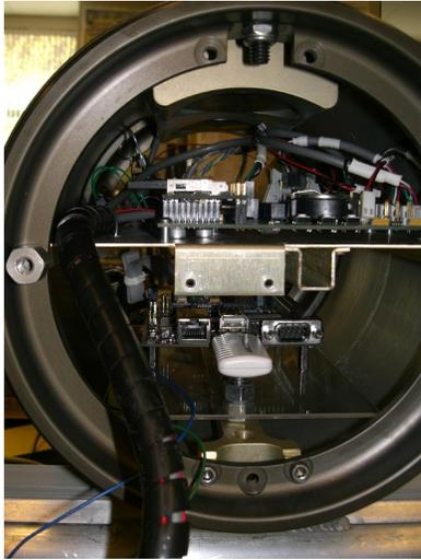
(a) An ARM-based TS-7800 Linux board. The new board is mounted in the lower half of the payload bay.
