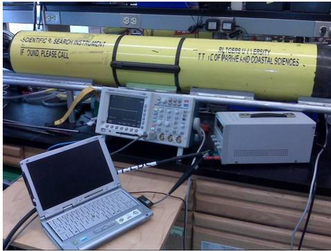
(a) Power Measurement Setup.
