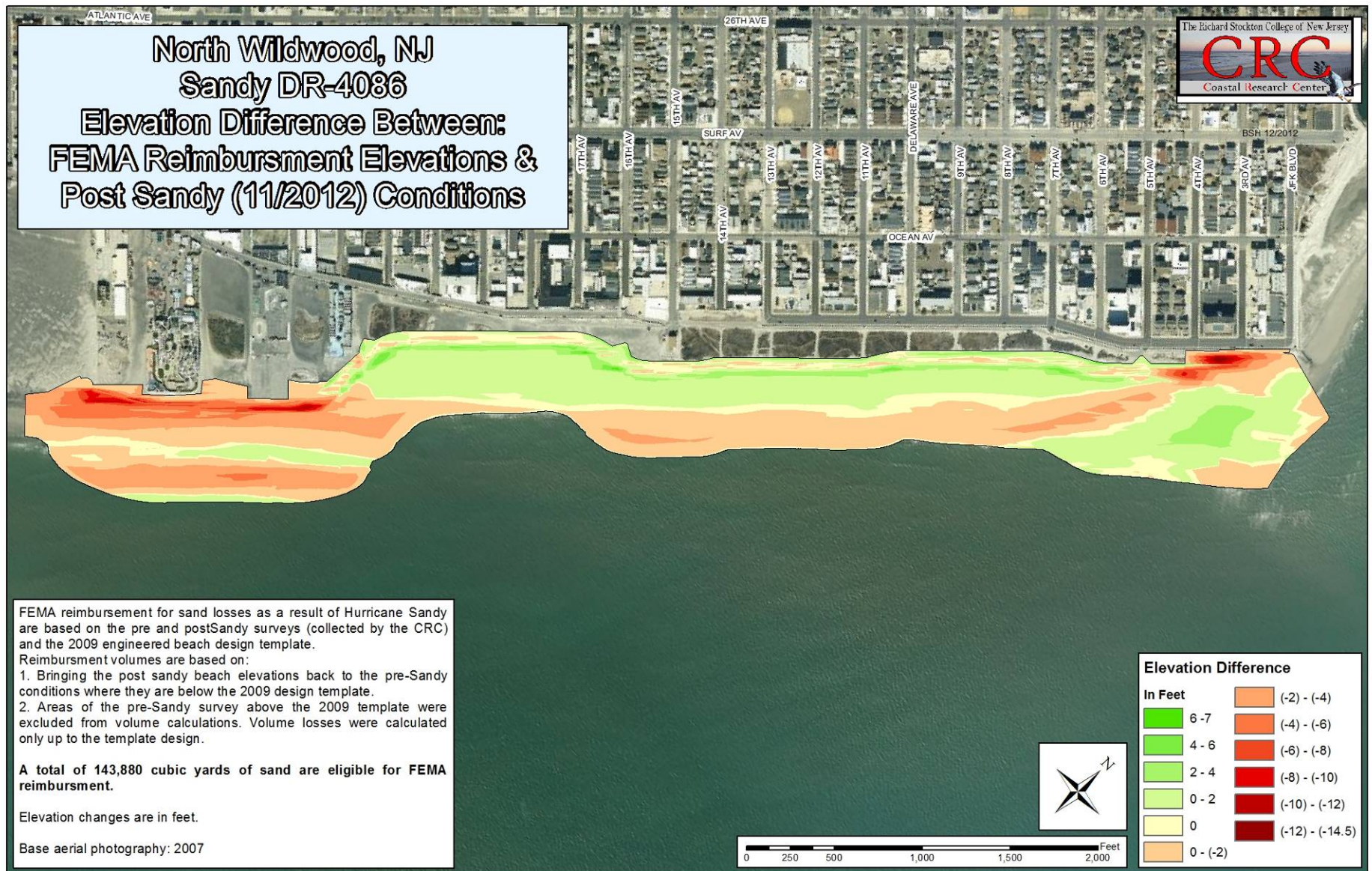
Figure 4. This map shows the elevation difference in lost sand volume due to Hurricane Sandy which is subject to FEMA reimbursement under DR-NJ-4086. Sand had accumulated along the middle of the municipal oceanfront beach above the design cross sections for this zone. FEMA will reimburse for loss to the project up to but not above the project's design conditions.
