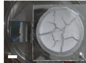
Figure C. 10 The effect of substrate wettability on the crack formation behavior of sample with initial thickness of Z_0 = 5 \text{ mm} and initial diameter of D_0 = 52 \text{ mm} as well as substrate with \theta \approx 30^\circ and temperature of: (a) T = 50^\circ \text{C} and (b) T = 60^\circ \text{C} . Each picture contains a portion of the side-view (left) and top-view (right) of the sample. Scale bar is 10 mm.
