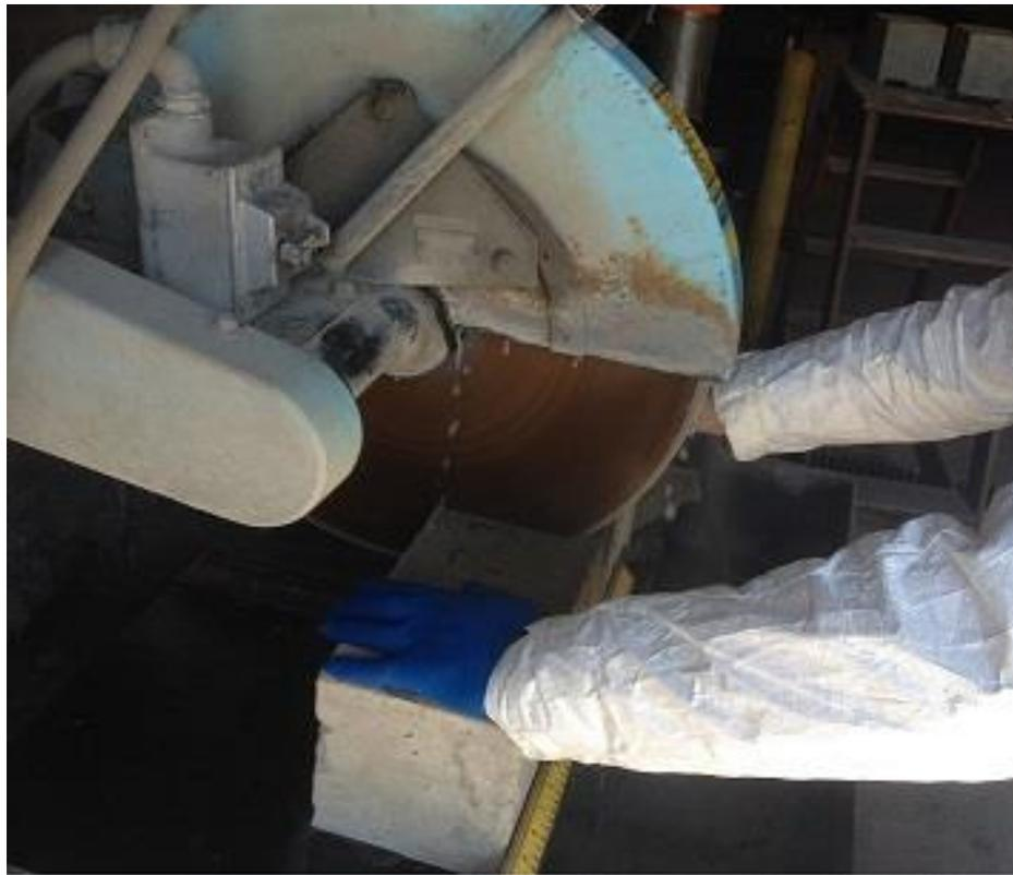
Figure 4. 4 Cut the concrete beams in the middle
