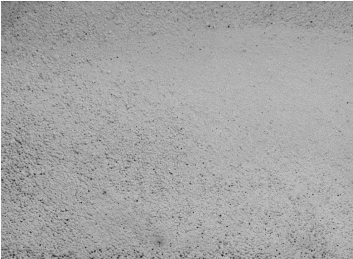
**Figure 2. 3 Autoclaved aerated concrete texture**
