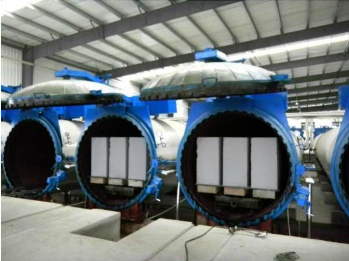
**Figure 2. 7 Autoclaved aerated concrete forming machine (www.diytrade.com)**
