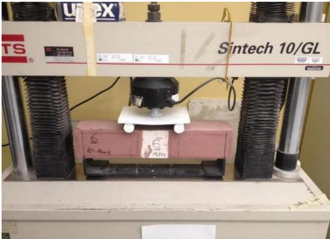
Figure 5. 11 Failure of AAC beams with five tows and shear enhancement.
