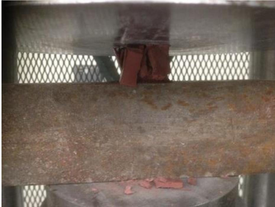
Figure 5. 6 testing of inorganic cubes in compressive machine
