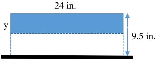
Figure A. 4 Cracked transformed section of the floor panel.
