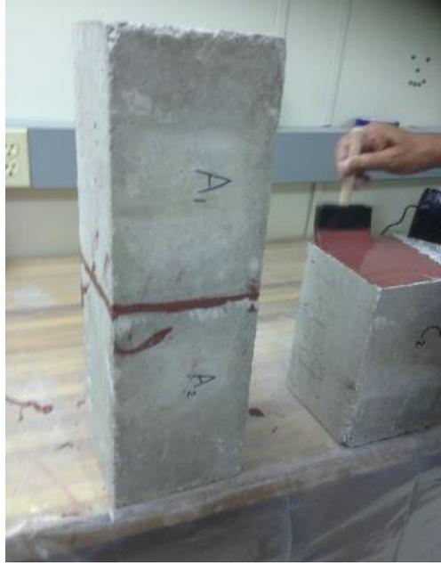
Figure 5. 1 Re-attached the cut concrete beams using inorganic matrix.
