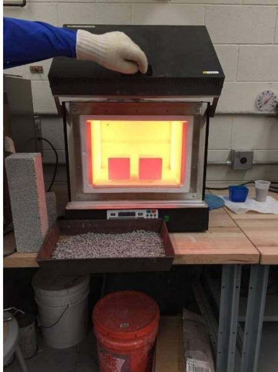
Figure 6. 7 (a). AAC cubes in the furnace at 1000 °C before being tested in compression
