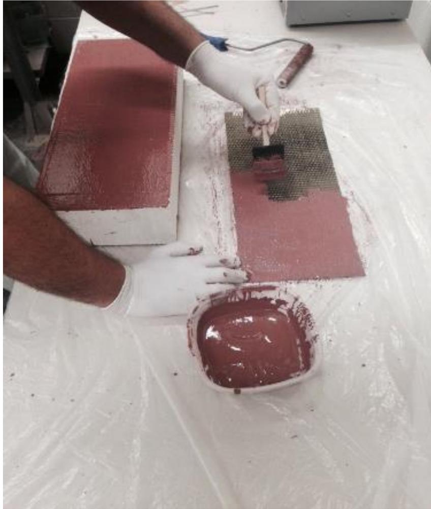
Figure 3. 11 Applying the inorganic matrix using hand lay-up technique
