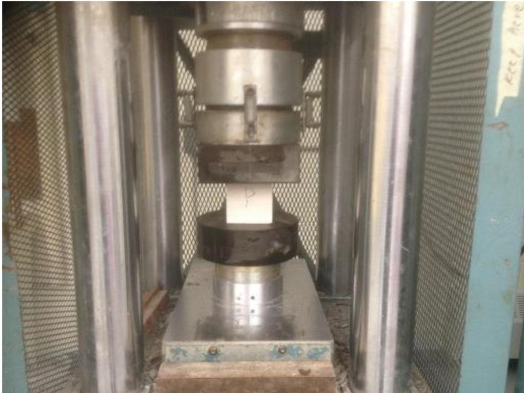
Figure 3. 2 Compressive strength setup for AAC.
