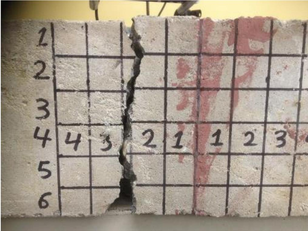
Figure 5. 3 Failure mode in cut attached faces concrete beams.
