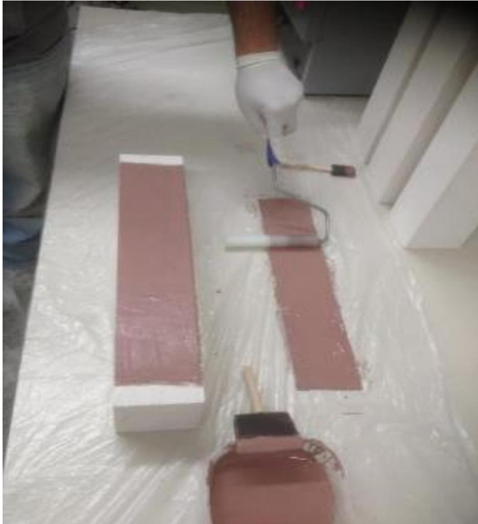
Figure 4. 2 Preparing and applying the inorganic matrix for AAC beams
