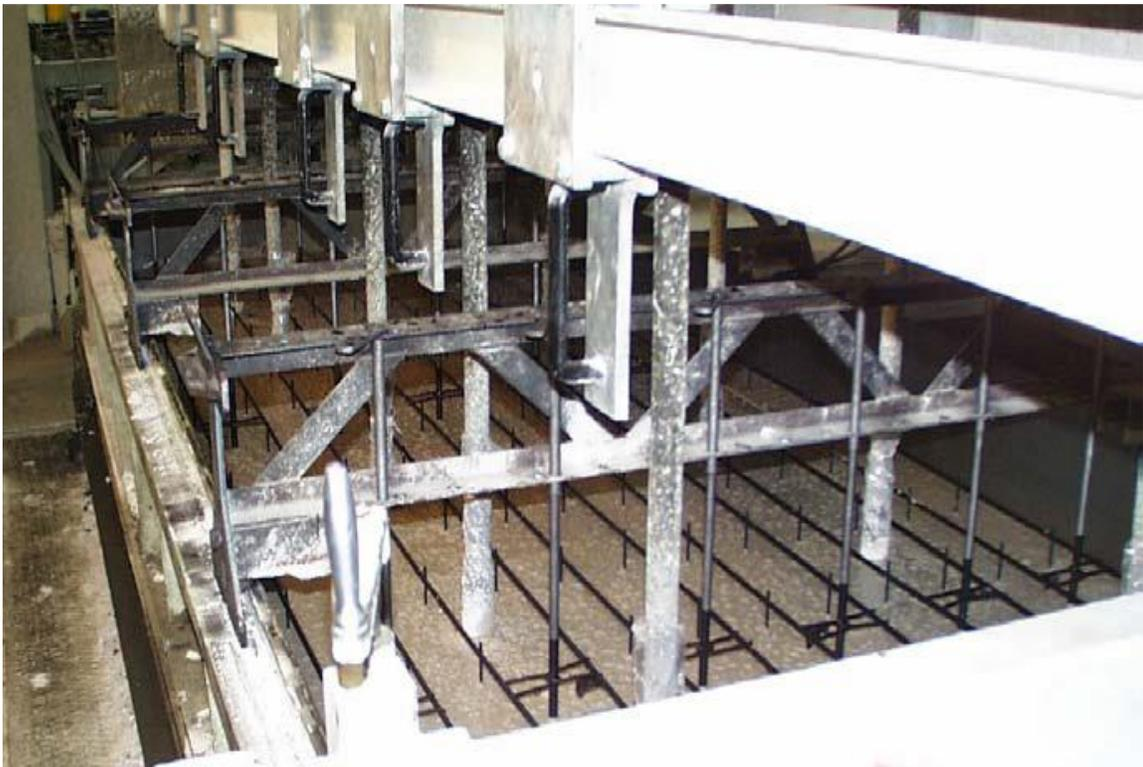
**Figure 2. 5 Autoclaved Aerated Concrete (AAC) mix in forms during the rising process (Tanner 2003)**
