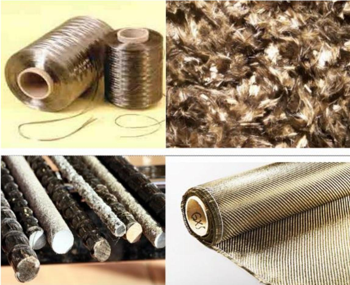
**Figure 2. 1 Variable types of basalt fiber (sudaglass.com)**
