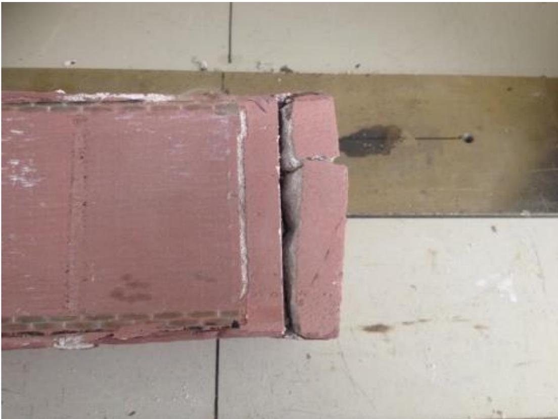
Figure 5. 14 Support crushing of specimen without U-wrap.
