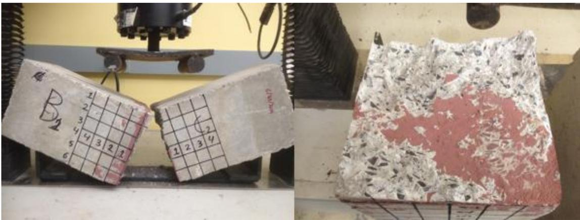
Figure 5. 4 Failure mode in cast attached faces concrete beams.
