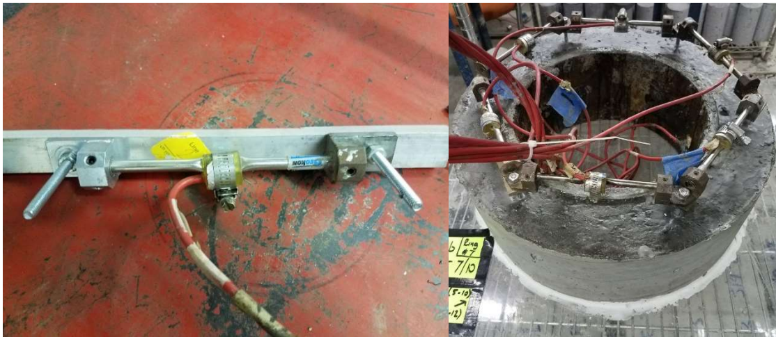
Figure 3.12 Typical Vibrating Wire with Plucking Coil and VWSG Ring
