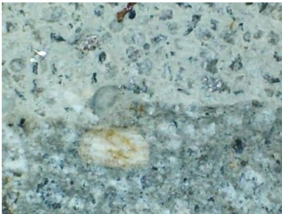
Figure 5.13 – Magnified x25 Interface of RSHPR and Substrate Concrete
