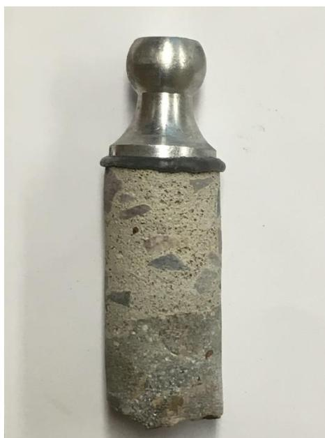
Figure 5.11 – Typical RSHPR & Substrate Pull Off Result
