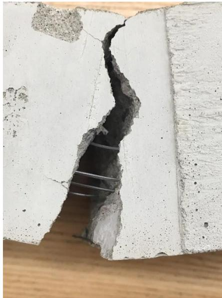
Figure 3.20 – Flexural Strength Fractured Specimen
