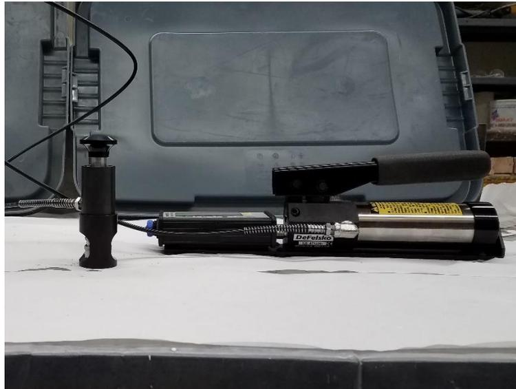
Figure 4.6 - PosiTest® AT-M Manual Adhesion Tester
