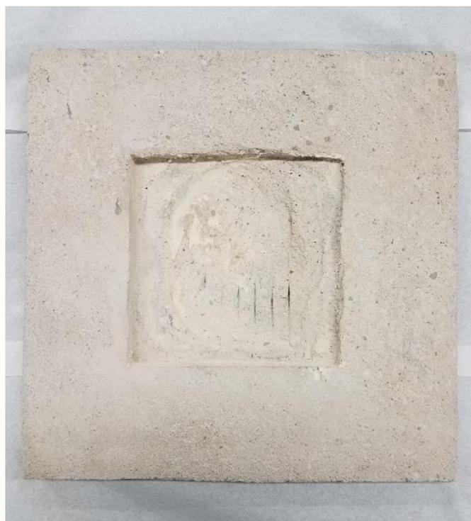
Figure 9.3 – Ferrocement Specimen with Simulated Damage Patch
