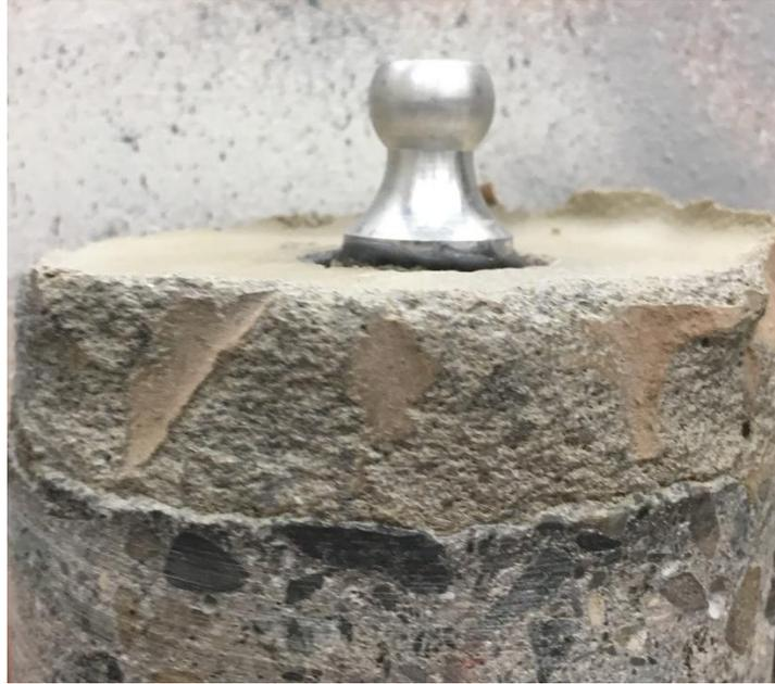
Figure 4.3 - 20-Millimeter Pull Off Dolly Attached to RSHPR Casted on Un-prepared Surface
