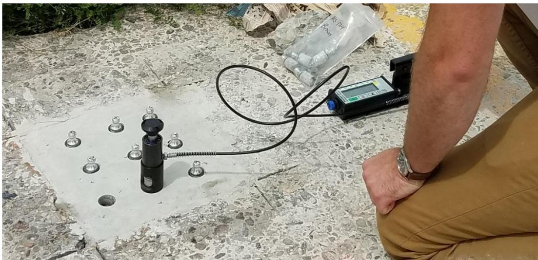
Figure 5.8 - Pull Off Test Conducted on Repaired Patch with a PosiTest® AT-M Manual Adhesion Tester
