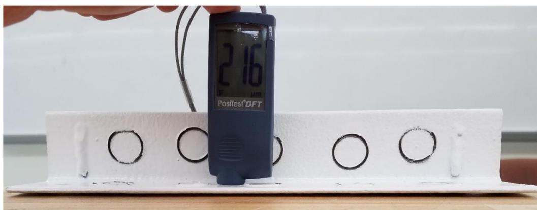
Figure 8.7 – Thickness gage used for measuring the thickness of paint layers
