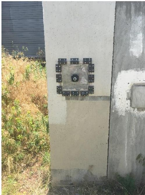
Figure 4.11 – Non-Horizontal Surface Repair: Patch Repair Test Set Up
