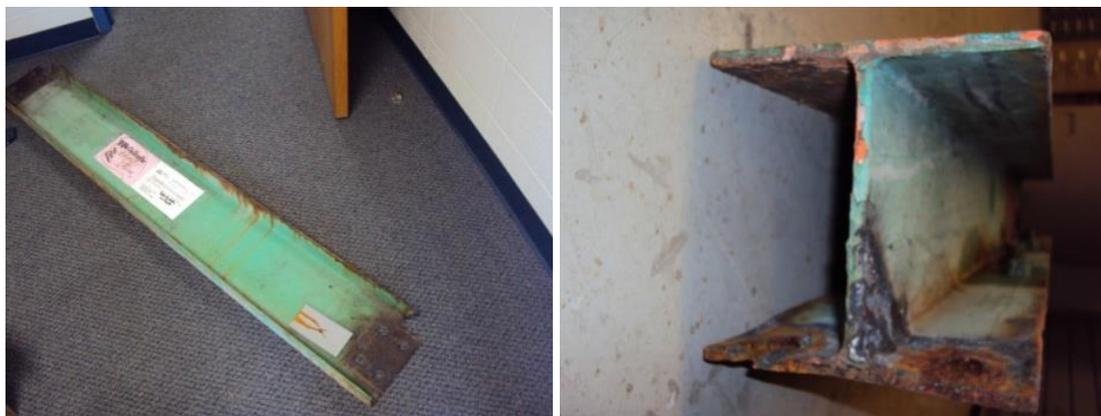
Figure 2. 6 – Typical Old Decommissioned Bridge Components
