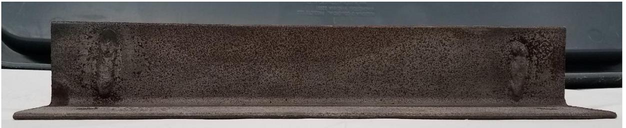
Figure 8.2 - Typical 1-inch-long welds on steel specimens
