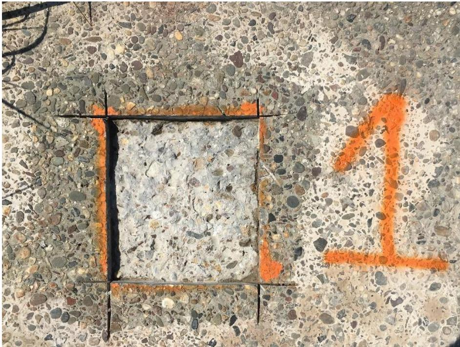
Figure 5.1 – Typical Simulated Patch
