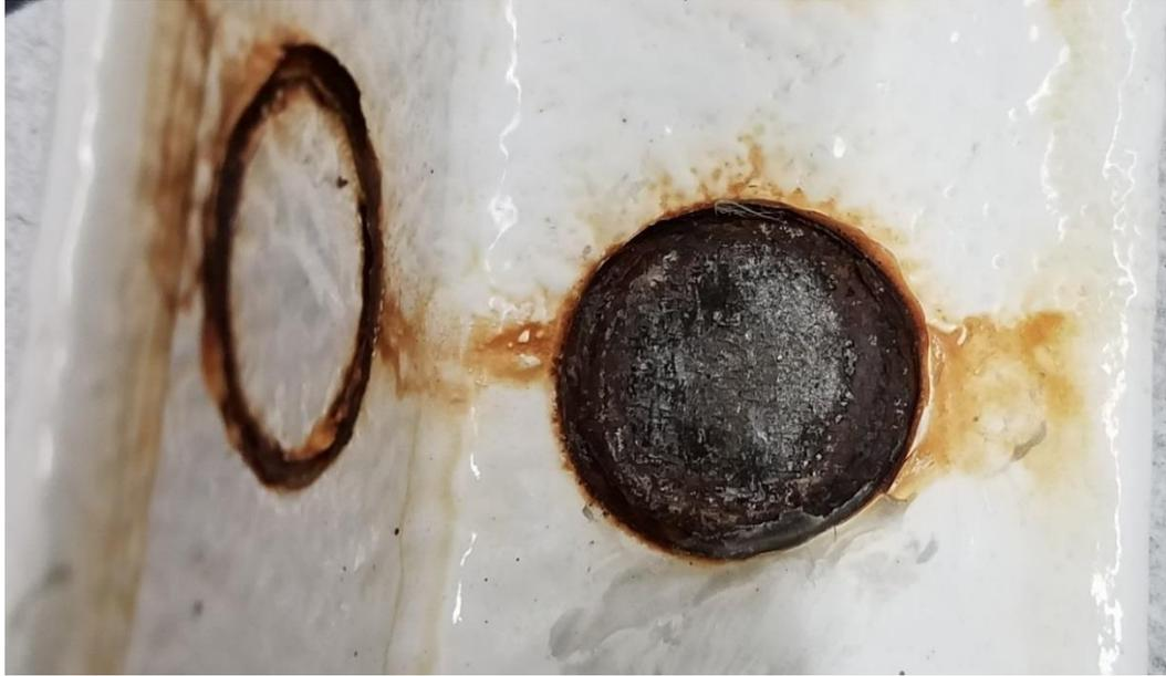
Figure 8.25 – Removed Paint After Pull Off Test
