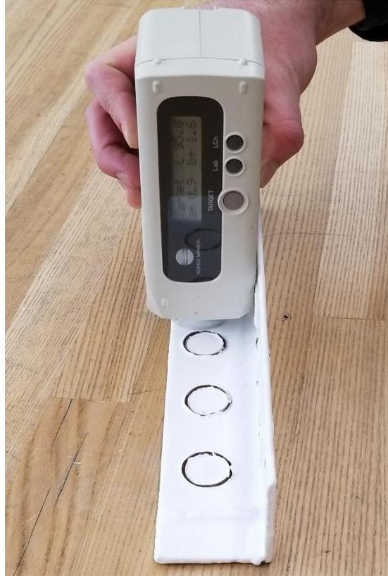
Figure 8.11 - Konica Minolta CR-10 Plus Color Reader
