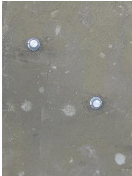
Figure 4.5 - Attached Pull Off Dollies on RSHPR Patch Repair
