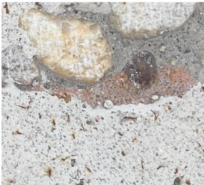
Figure 9.14 – RSHPR Patch Repair: 10 Months After Placement Interface
