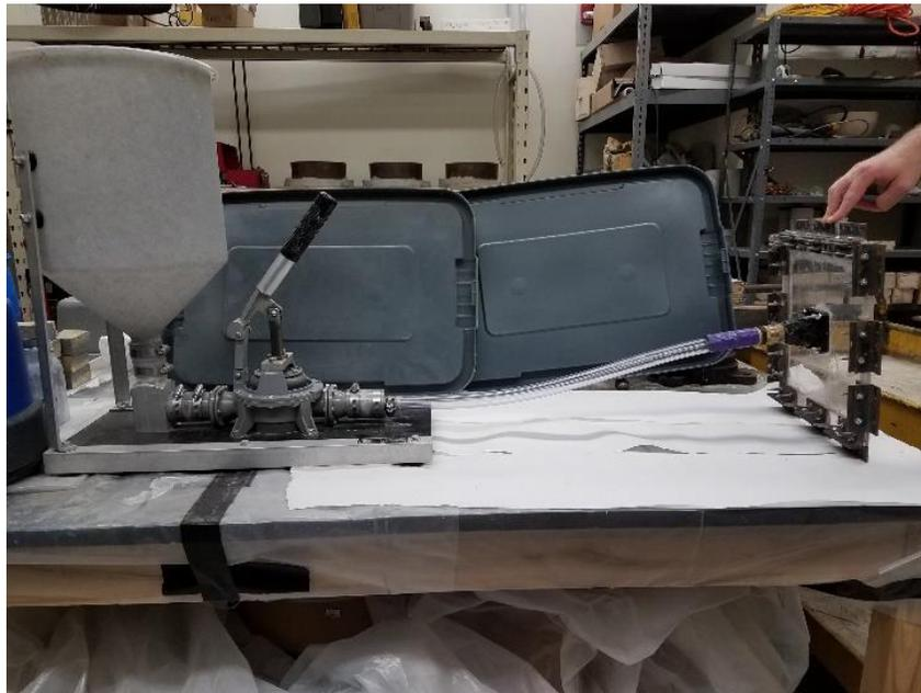
Figure 4.9 – Non-Horizontal Surface Patch Repair Application System
