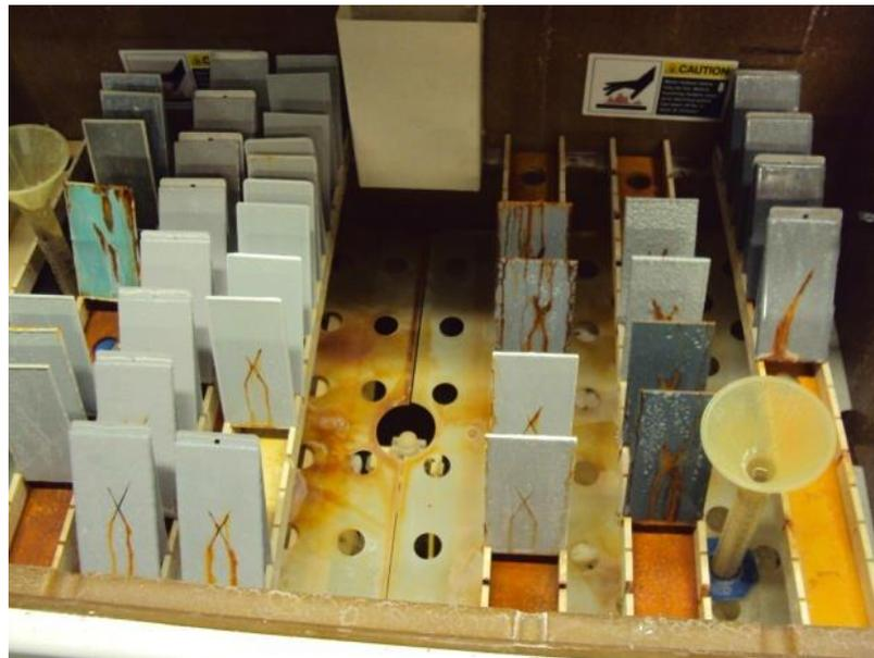
Figure 2.4 - Typical Salt Fog (Corrosion) Test Set Up with Scribed Samples
