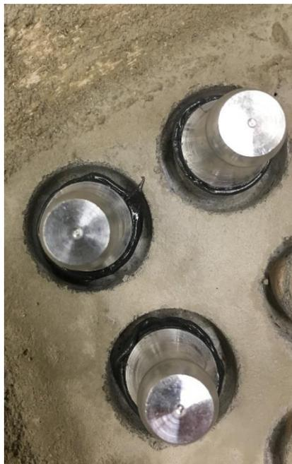
Figure 9.5 – Pull Off Dollies Epoxied on a Rapid Set Repair Durability Specimen
