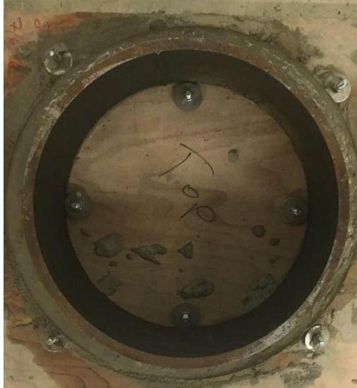
Figure 3.17 – Restrained Shrinkage Ring Sample
