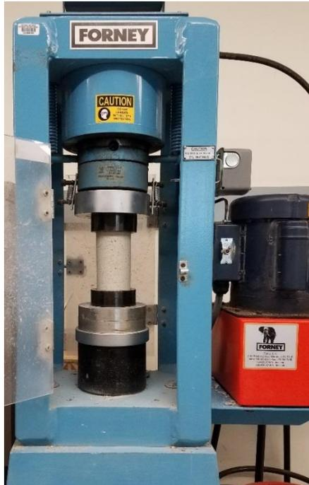
Figure 3.12 – RSHPR Compressive Specimen in the Forney 250-Kip Compression Machine
