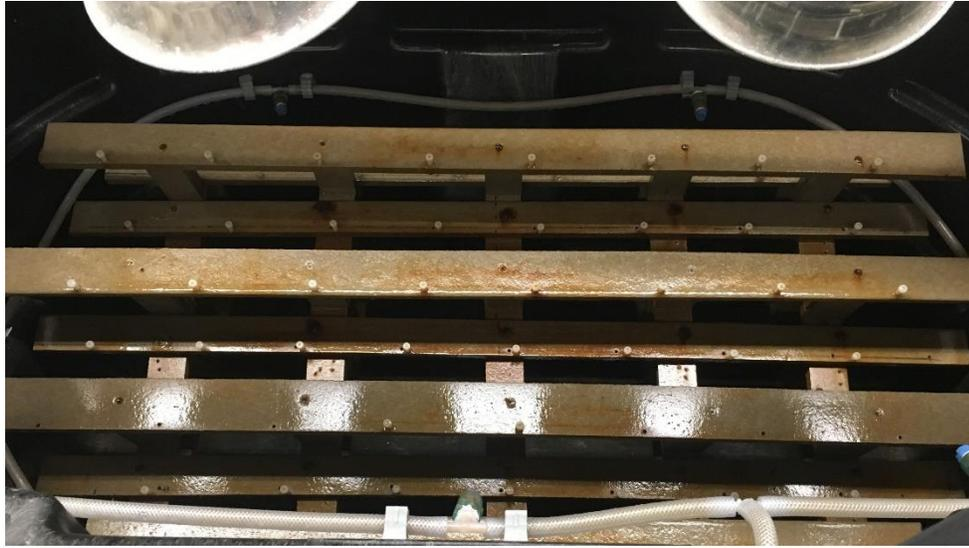
Figure 7.6 – Specimen Holding Rack
