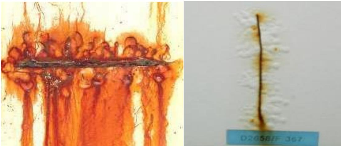
Figure 2.5 - Scribe cuts on painted steel specimens ready for evaluation
