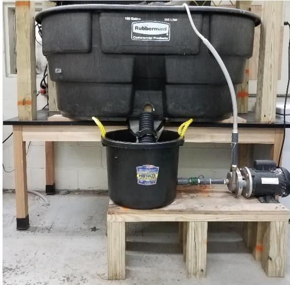
Figure 7.1 - 150 Gallon Polyethylene Plastic Tub and Salt Water Solution Reservoir
