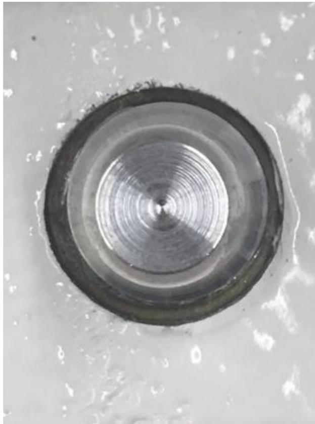
Figure 8.9 – 20 Millimeter Pull Off Dolly: Epoxied to Thin Coated Steel Specimen
