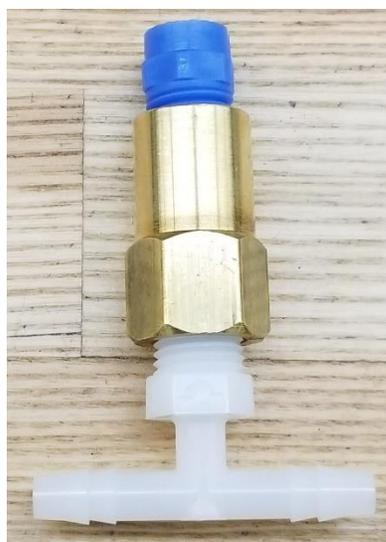
Figure 7.5 - Salt Water Sprayer Assembly
