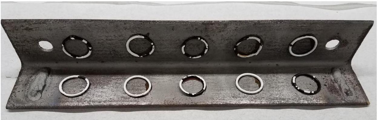
Figure 8.3 – O-rings attached to steel specimen
