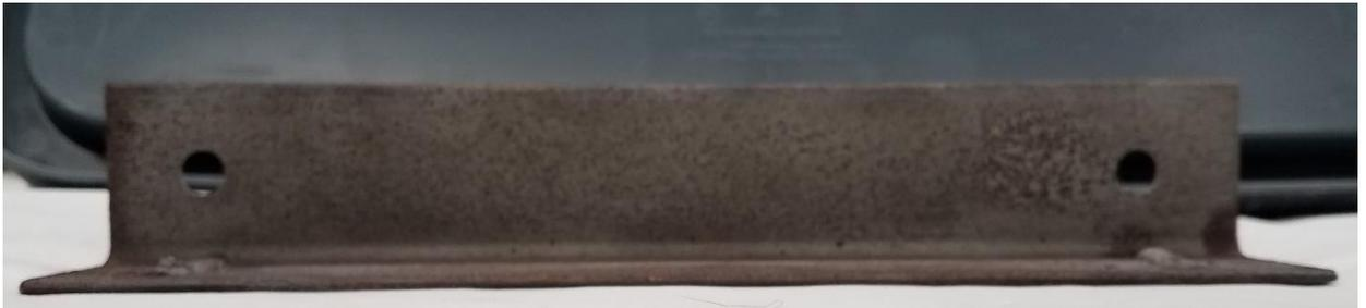
Figure 8.1 – Typical ½ inch diameter holes in steel specimens
