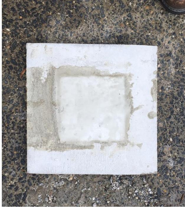
Figure 9.4 – RSHPR Durability Specimen After Simulated Patch Repair
