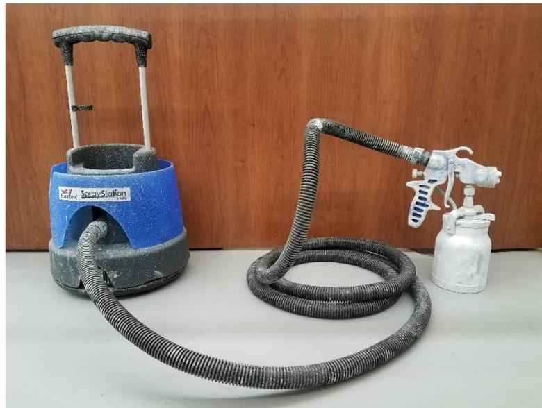
Figure 8.5 – Low Pressure Spray Apparatus
