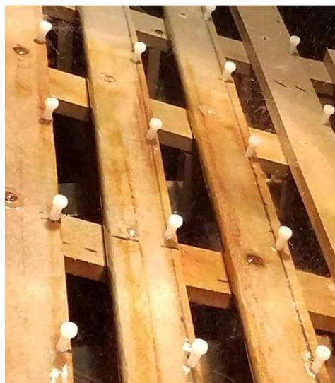
Figure 7.7 - Shoulder Screws Installed on the Specimen Holding Rack
