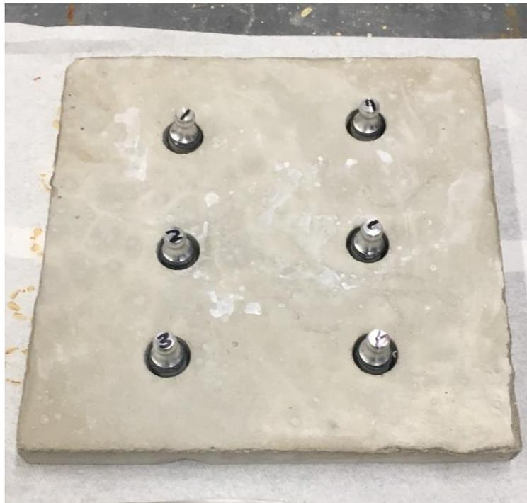
Figure 4.2 - Laboratory RSHPR Slab with attached Pull Off Dollies
