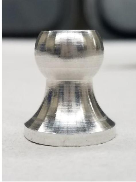
Figure 4.4 – 20-millimeter Pull Off Test Dolly
