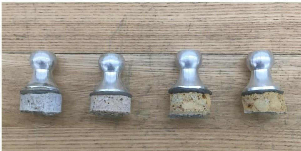
Figure 9.11 – Typical Pull Off Specimens
