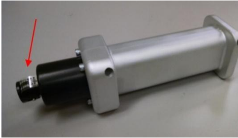
Figure 9 - StrikeVEMP striker, red arrow points to internal FSR sensor at the striker tip
