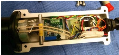
Figure 8 -Internal of the StrikeVEMP striker, including the metal pin, spring, FlexiForce board, and switching circuit (from left to right)
