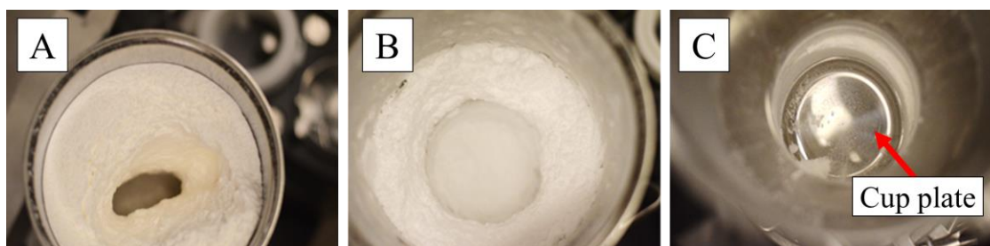
Figure 44. Top view of the refill unit, looking downwards from the hopper. (A) Arching observed for cellulose, (B) arching observed for acetaminophen (C) view of the hopper unit when empty.
