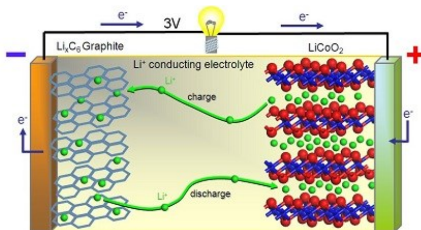
Figure 1-3: A diagram explaining the operation of a Li-ion battery that consists of a graphite based negative electrode, and a \text{LiCoO}_2 positive electrode. 10
