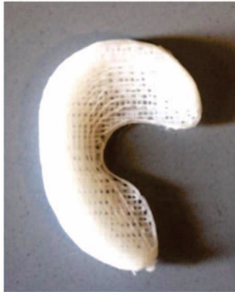
Figure 14 Lee et al. FDM printed PGA/PLA microspheres, PCL meniscus scaffold 69 .
