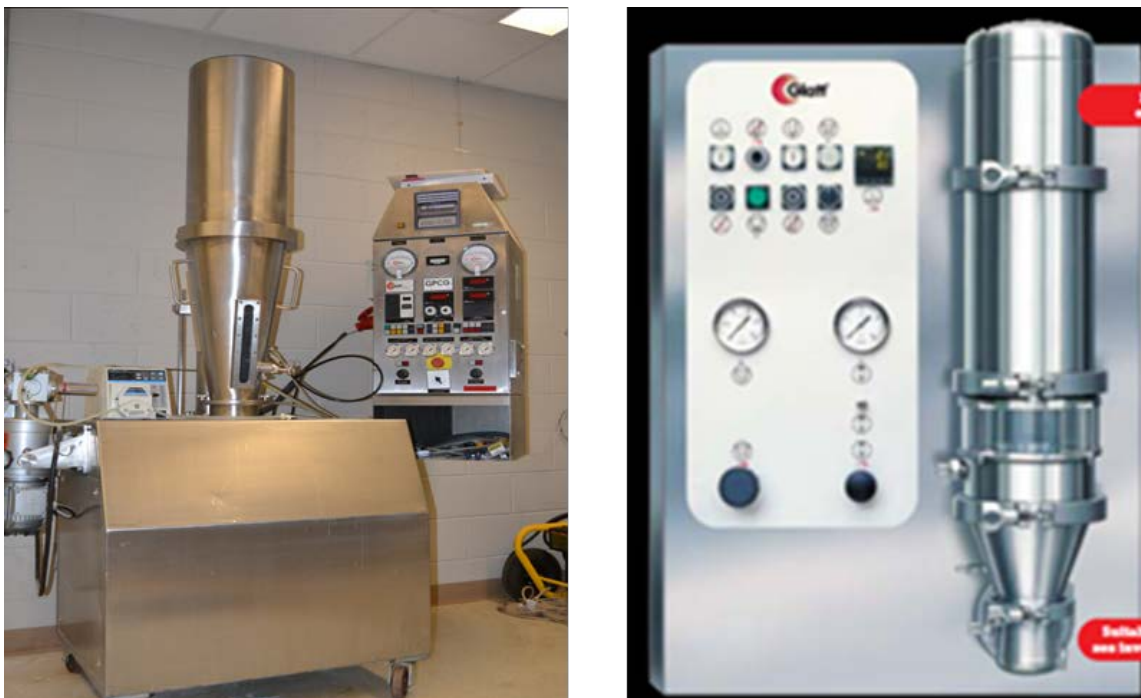
Figure 2-3: Fluidized bed dryers chosen for impregnation development: Glatt GPCG 1 - 3kg scale (left) and Mini Glatt – 500g scale (right).
