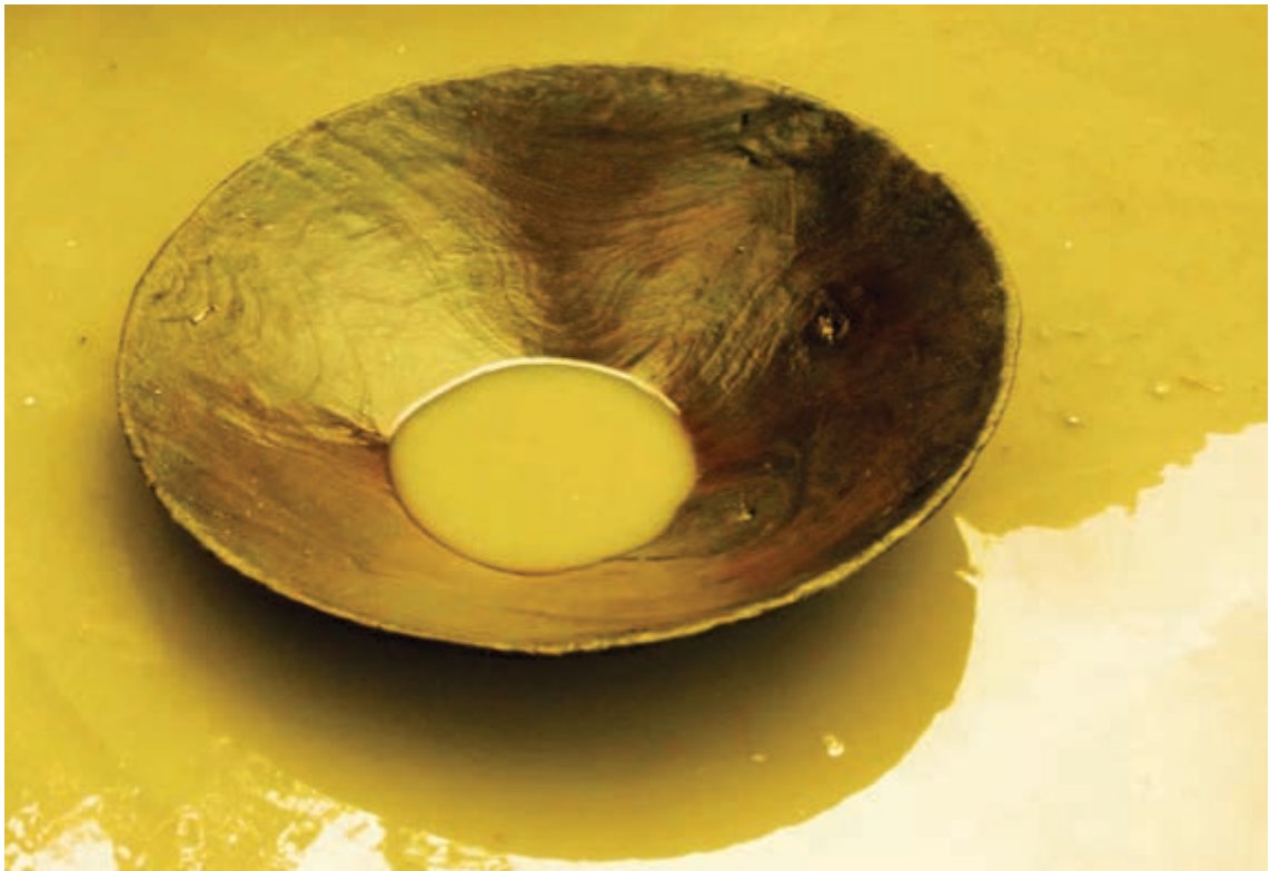
Figures 5 and 6. A miner was carving this wooden batea when I stopped to visit him. He told me that most important thing was to choose the right wood: “it should be of good quality, never to twist or crack, even if it is kept in the water for a long time and then left under the sun for the rest of the day.” One of the woods used for bateas is classified as Laure-cacho ; close in strength to Oak. Photographs by the author.
