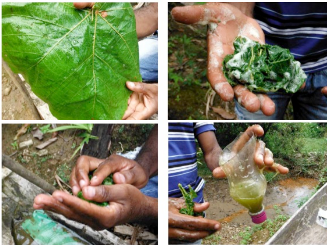
Figure 43. Malva leaves ( Hibiscus furcellatus ) used to separate alluvial gold from the waste material in the “green gold” process employed in the Chocó Department, Colombia. Source: Brooks, W.E., Sierra-Giraldo, J.A. and Palacios, F.M. (2015) “Green Gold—Dirty Gold, Tadó, Dept. Chocó, Colombia.” In: Natural Resources , 6, 534-542. http://dx.doi.org/10.4236/nr.2015.611051 (accessed January 8, 2017).
