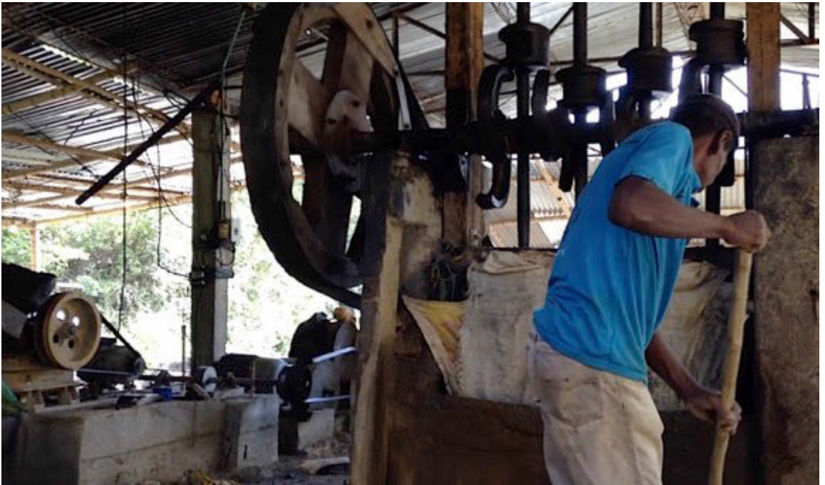
Figures 11 and 12. Above, the entrance of a mining tunnel in Mindala. In the picture below an old molino de pisón [Californian stamp mill] is shown. Here iron bars crush rocks imbibed in water in a rhythmic compass whose sound is both exciting and macabre. Tarps or sacks are used as filters for the particles. Photographs by the author.
