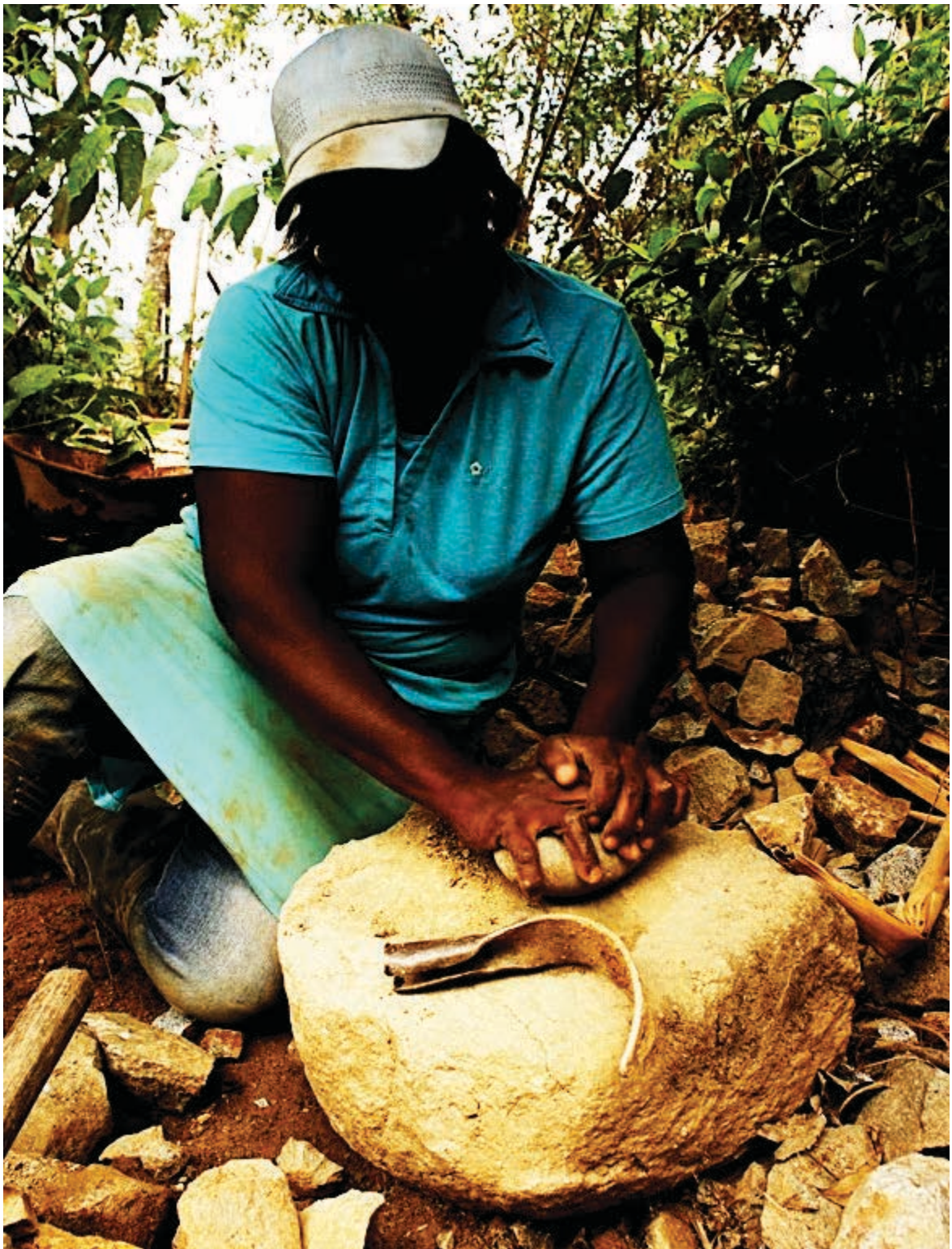
Figure 3. Bertha's mining technique. In the lower part of the image, the almocafre tool, described in the text, is shown. Photograph by the author.
