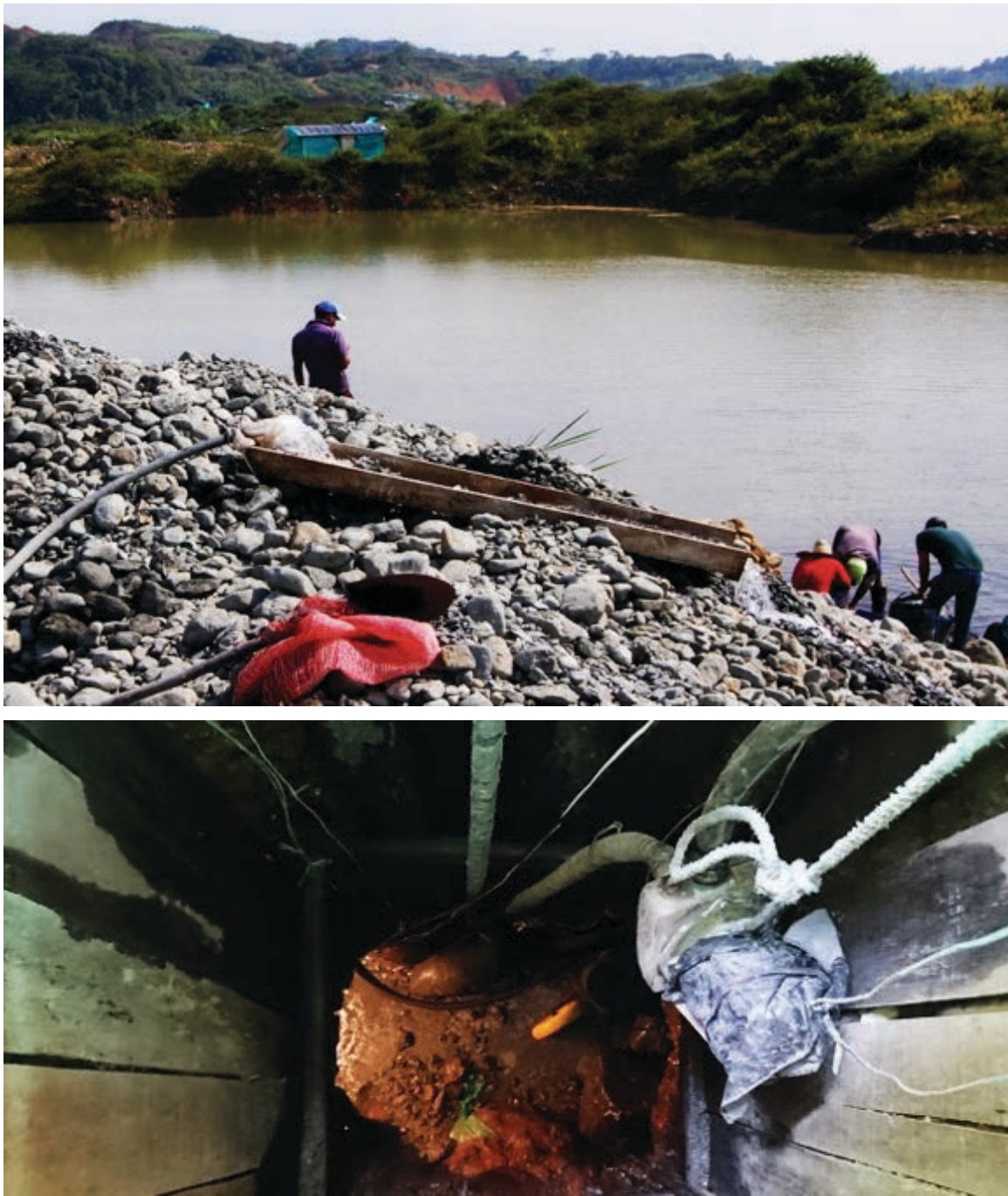
Figures 41: Cúbicos in the Quinamayo River. The name is after the shape and type of the tunnels used, which go down in a vertical line extracting cubic meters of lodes and rocks near the riverbanks. In one of this cúbicos visited on May 2015, I found 9 people working inside the mine, which was being drained with motores de achique [pumps] because the river was increasing the water pressure on the tunnels. Below the mountain of rocks eight barequeros were allowed to search for ore particles after the clasificadora had remove the most valuable rocks and lodes that were later taken to the long rows of tumblers that crush minerals. Photographs courtesy of Laura Silva Chica.
