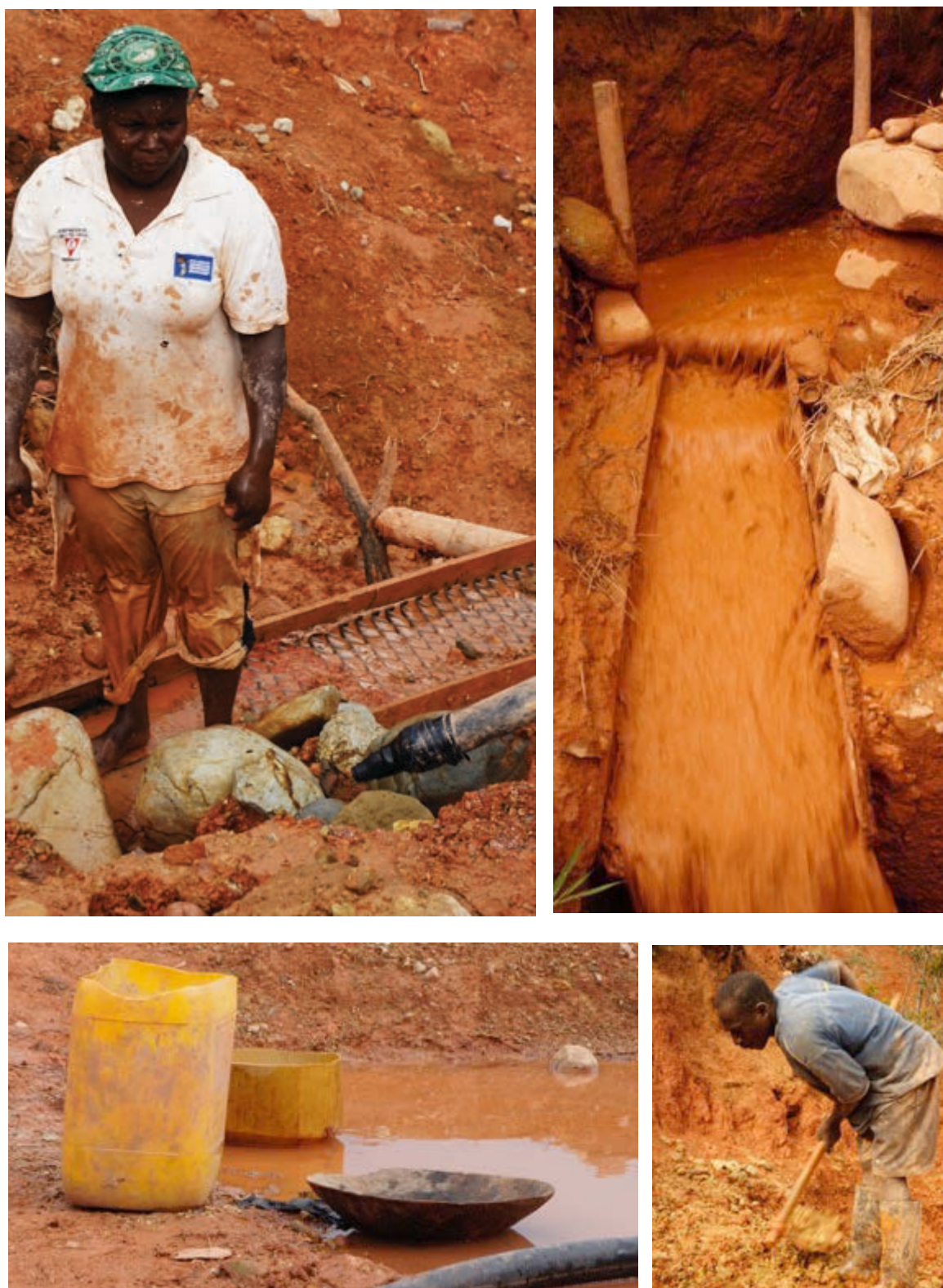
Figure 8. Ground sluicing miners in La Toma, Suárez. Photographs by the author.
