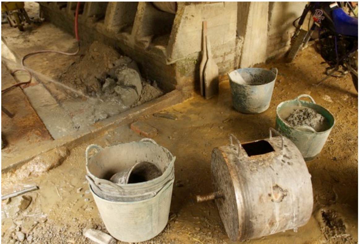
Figure 44. Planta de beneficio with spinning iron tumblers designed to help separate gold. As know as Cocos these tumblers and its technique arrived to the area in 2004 brought by miners from Antioquia. Tumblers are filled with water, rocks, lodes, iron spheres, and liquid mercury. Once the rocks are reduced to mud, miners wash the remaining lodes in large canals where the gold, trapped by mercury, remains in the bottom. Then the amalgam between gold and mercury needs to be taken to refineries or furnaces where the mercury is evaporated setting the gold free.
