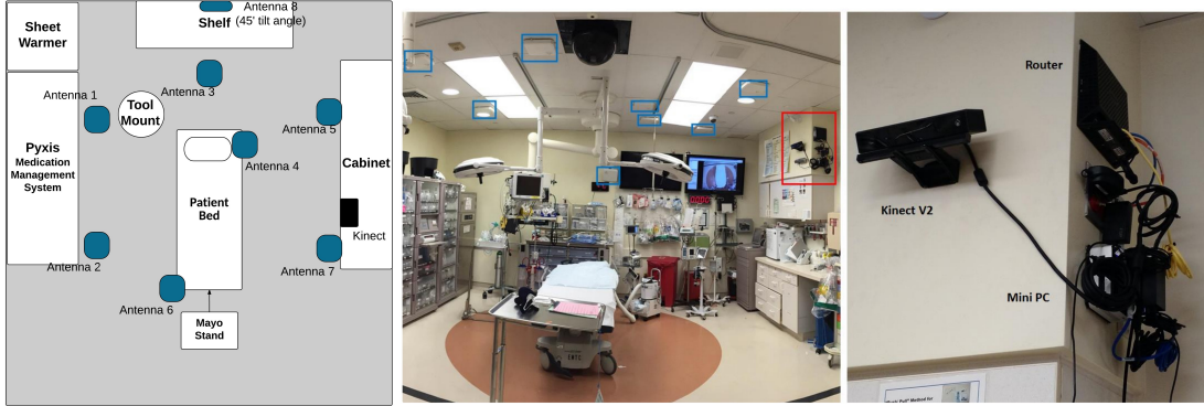
Figure 4.5: Left: Antennas 1 to 7 are mounted on the ceiling and facing down; Antenna 8 is mounted on the wall and facing 45° to the ground. Middle: A photo of the room with the antennas labeled with blue rectangles and the Kinect and Mini PC labeled with a red rectangle. Right: Zoom-in of the Kinect, router, and Mini PC.
