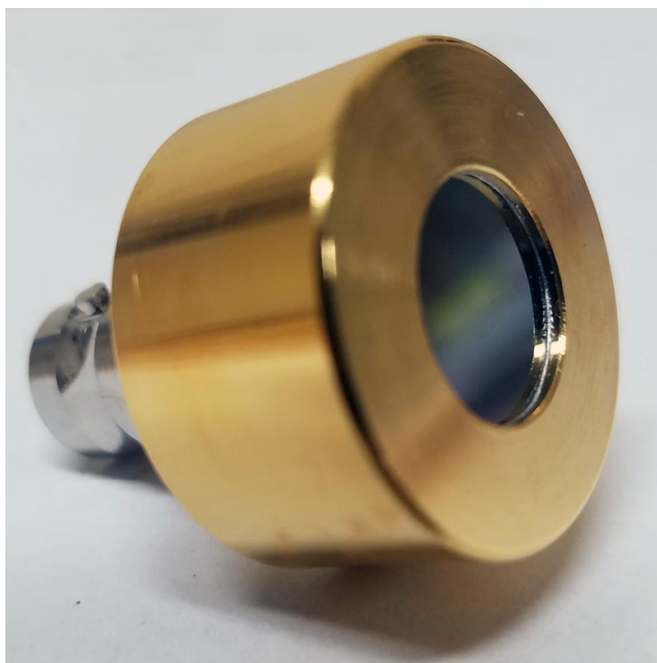
Figure 3.2 Commercial depleted Si detector from Ortec 30 , commonly used for RBS and high-energy particle detection.
