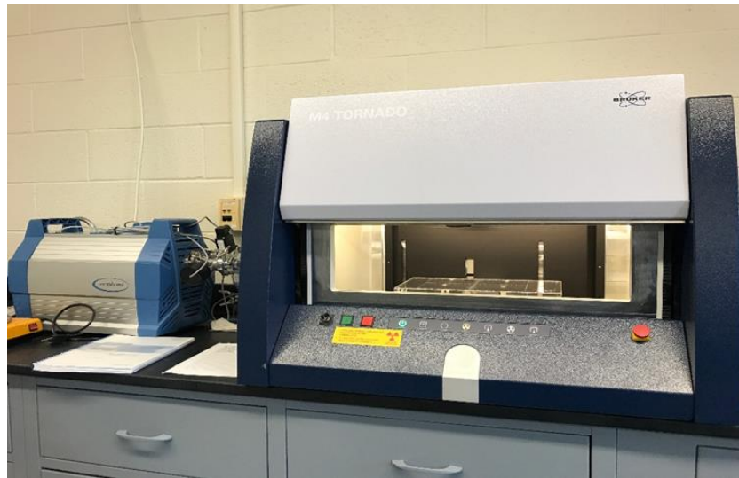
Figure 10 : M4 Tornado micro-X-ray spectrometer by Bruker accompanied with a vacuum pump
