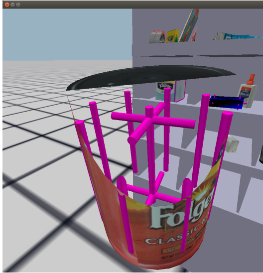
(a) Grasp descriptors for parallel end-effectors.
