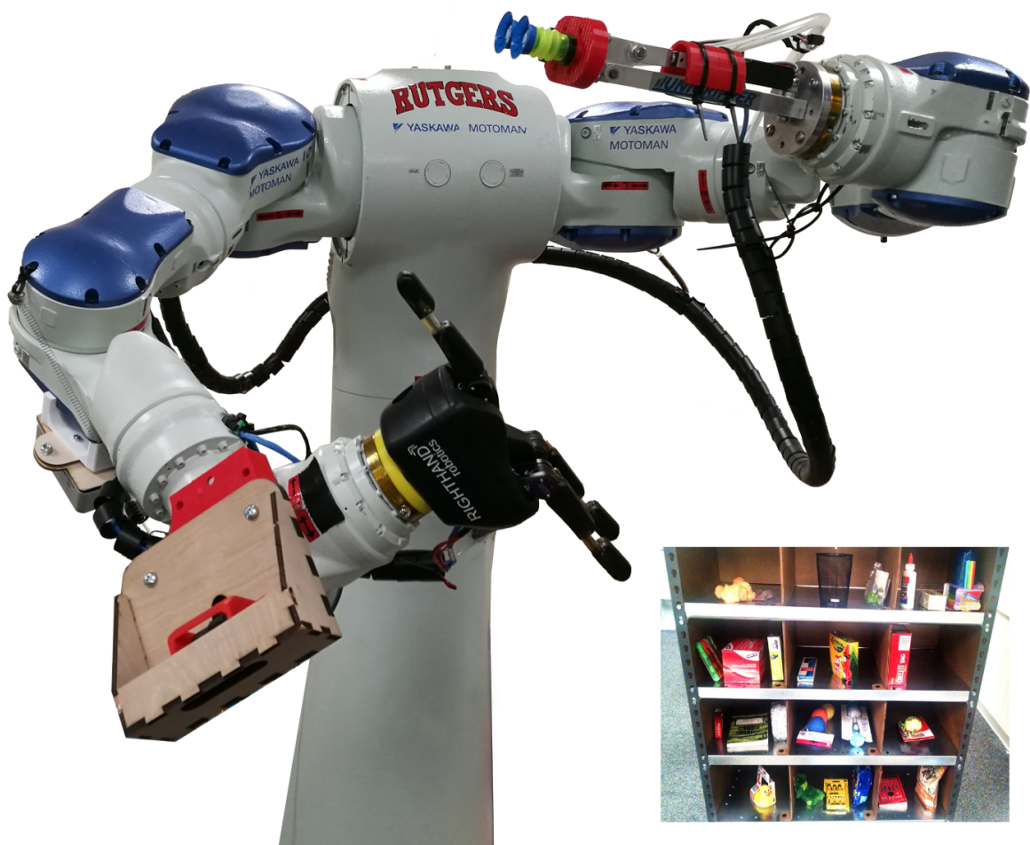
Figure 2.1: Hardware setup evaluated for warehouse picking.
