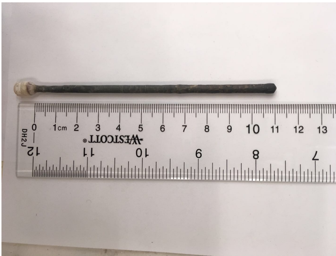
Figure 3.1: A photograph of the as-grown Sr_3Sn_2O_7 single crystal boule.
