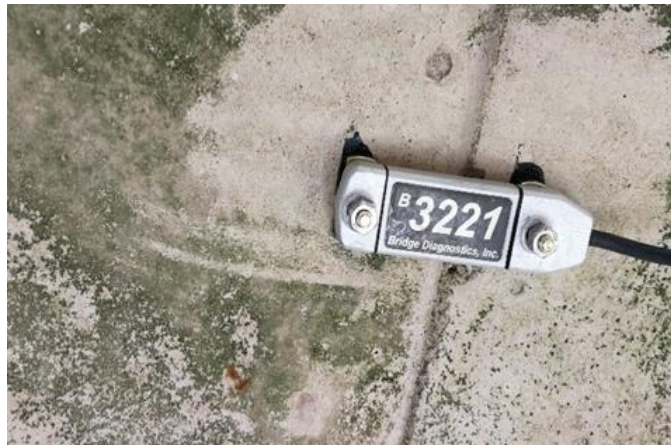
Figure 6. STS Strain Transducer Installed on a Bridge Superstructure Member
