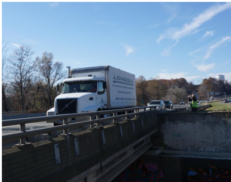
Figure 13. Diagnostic Load Test
