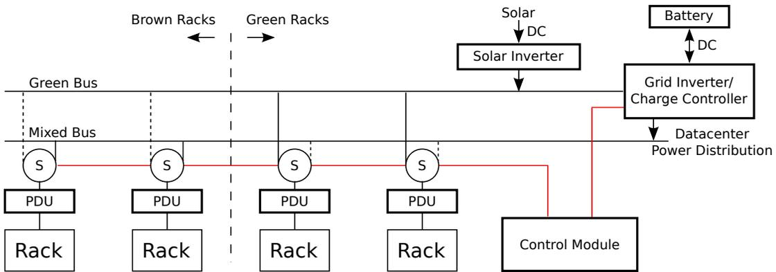
Fig. 1. Power distribution infrastructure. The vertical dash line shows an example partitioning of the racks into a brown part (where racks are switched to the Mixed Bus) and a green part (where racks are switched to the Green bus) by a scheduling policy. This scheduling is discussed in Section IV.
