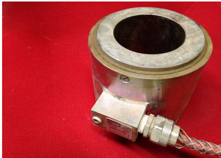
Fig 3.29 Typical Load Cell Used to Monitor Applied Load
