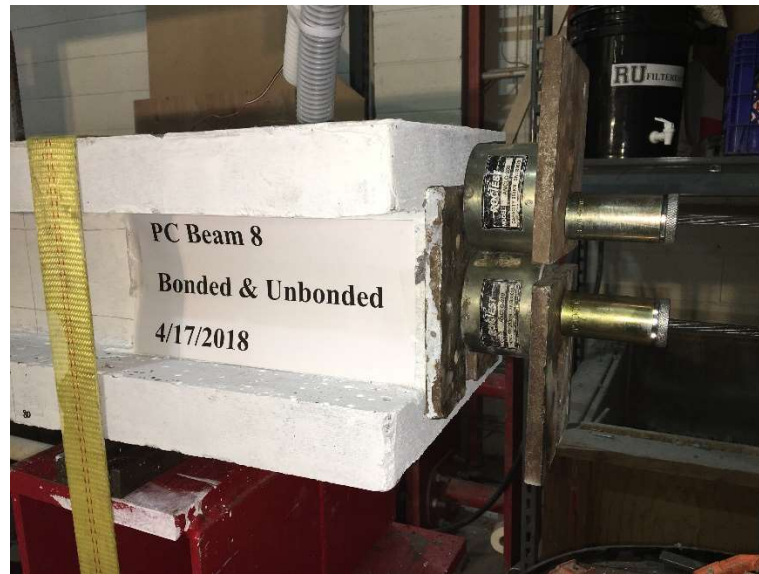
Fig 3.30 Typical Load Cell Used with Bonded and Unbonded Tendon
