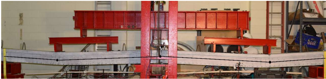
Fig. 4.3 Plastic Hinges Locations for Third-Point Loading
