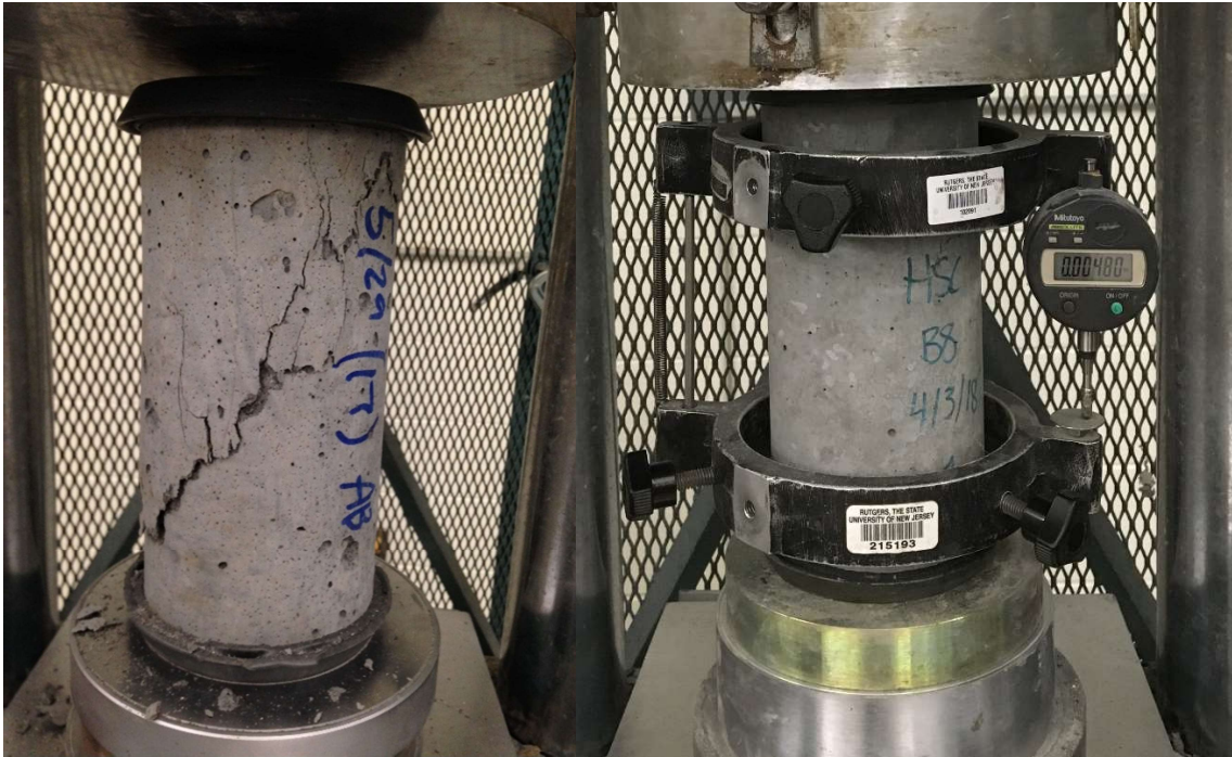
(a) Compressive Strength Test Setup
