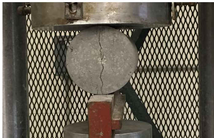
(c) Splitting Tensile Strength Test Setup
