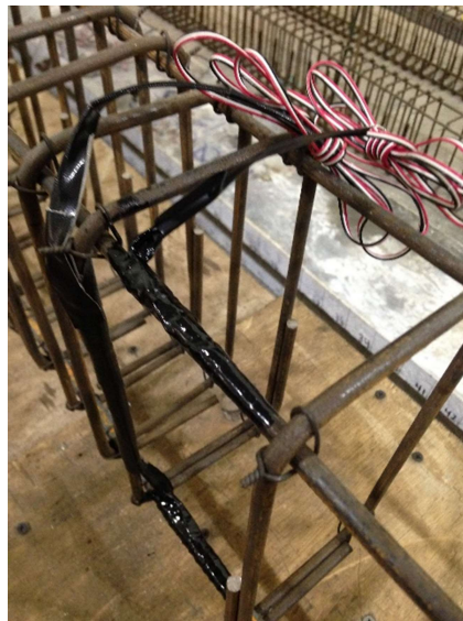
Fig 3.33 Strain Gauges installation in the Longitudinal Steel
