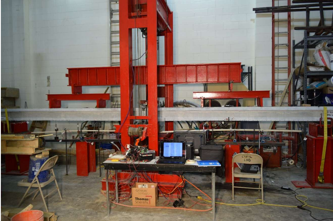
Fig 3.36 New Loading Frame Setup and Beam Test
