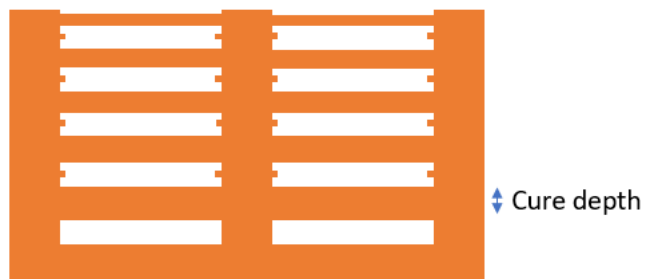
Figure 2.9 Bridge structure illustration for cure depth measurement
