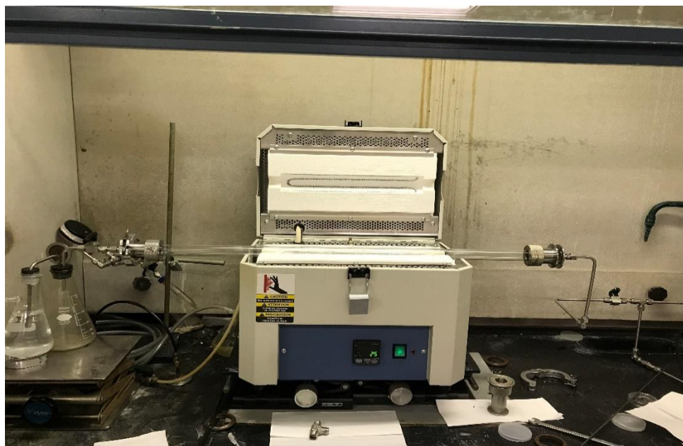
Figure 52 The new single-zone furnace was used for CVD \text{NbS}_2 growth. Even though it has relatively a smaller temperature zone, the higher (1250 ^\circ\text{C} ) temperature can be reached at.
