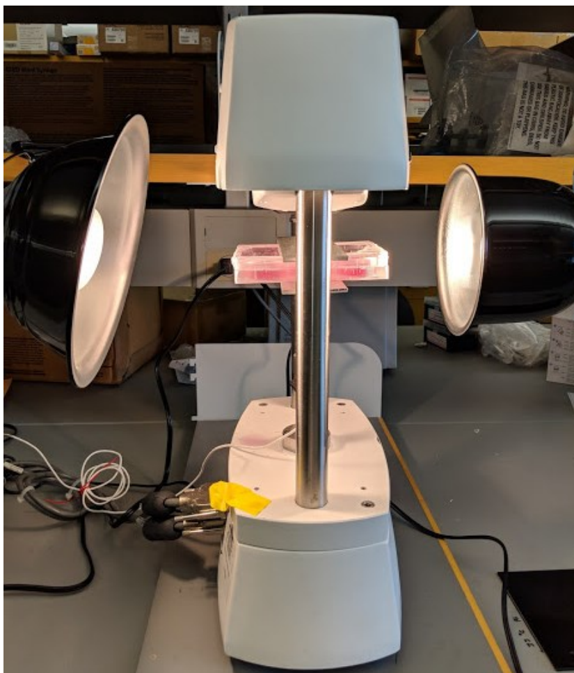
Figure 2.6: Set-up of the Electro Force Instrument (Bose-3100) used in the stimulation protocol for RN33B cells. Well plates are stacked, wrapped with parafilm to prevent infection, and the neurons were maintained at (33 and 37) °C due to their sensitivity to temperature.
