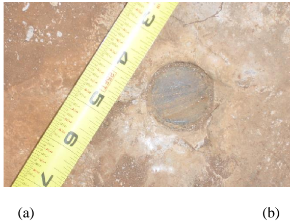
Figure 2.16 (a) Failure of cantilever sign support and (b) fractured anchor bolt (Ian, 2009)
