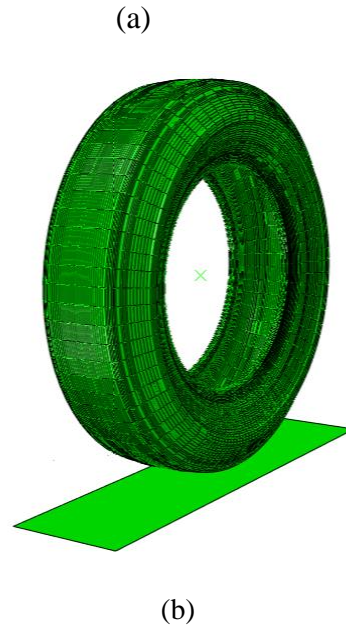
Figure 4.13 ASTM standard E524 smooth tire: (a) tire section (ASTM 2005b); (b) 3D tire-pavement interaction model
