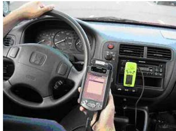
Figure 3: EZCab driver system consisting of an HP iPAQ equipped Orinoco 802.11 wireless card and Geko 201 GPS receiver
